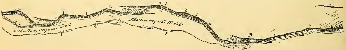
FIG. 1. Map of a zone of dislocation revealed at the surface after the earthquake in the Owens Valley, California, in 1872. Surveyed by Mr. W. D. Johnson, U. S. Geological Survey, in June, 1907. Scale, 240 feet equal one inch. The figures indicate throws, and the arrows the facings of the scarps.
