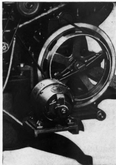
Detail of Motor Drive Showing—Motor, Support and Combination Gear and Pulley
