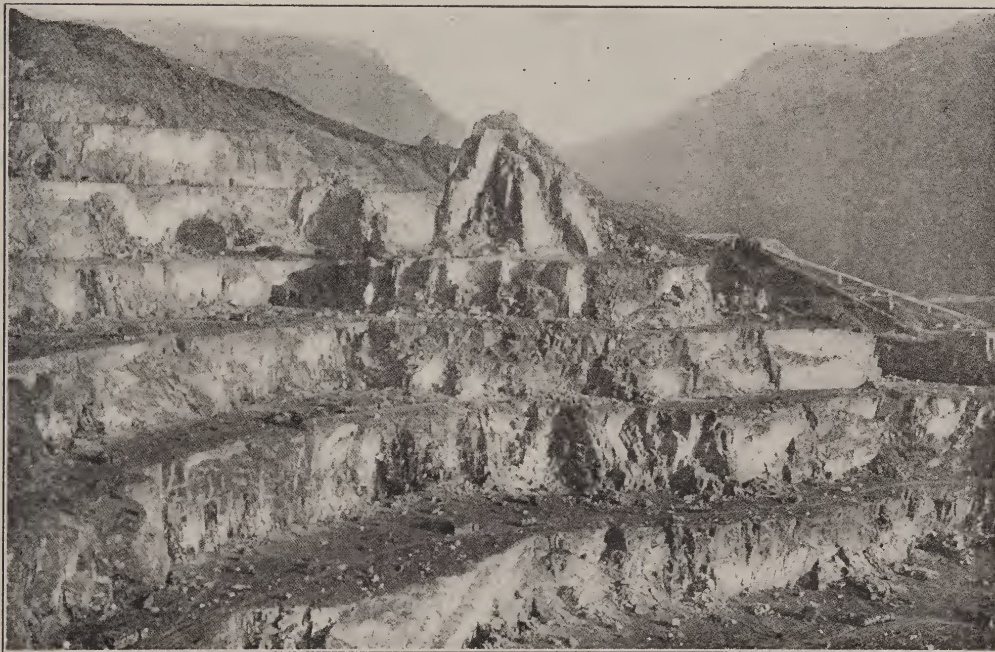
Galleries showing great Slate Quarry at Port Dinorwic, North Wales, which has been worked for two hundred and fifty years, but only during the last century has the slate been quarried systematically. The galleries are each 75 feet high and 3,000 persons are employed in the quarry.
