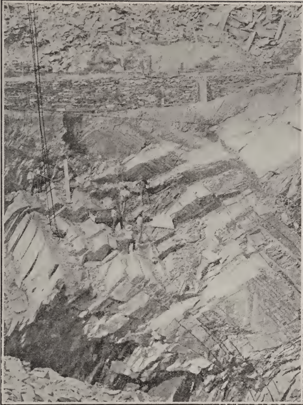
Workmen clearing away the debris and ribboned slate in a quarry near Slatington, Pa., in order to reach a thick workable bed of valuable slate. This condition does not exist on the Peach Bottom ridge.
