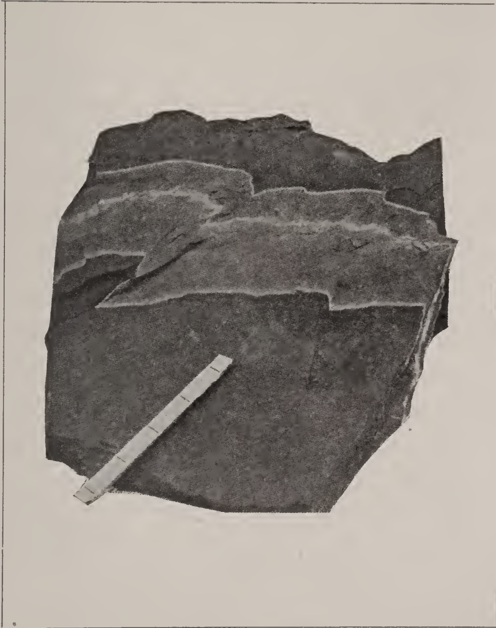
A ribboned slate from a quarry near Hatch Hill, in Whitehall, New York. Ribbons are seldom found in the best quality slates and are not of the same hardness as the marketable product.
