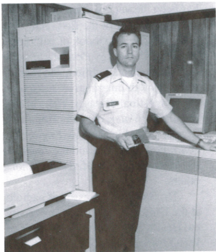
ILT Joseph Healey, MS, USA, AMS Deputy Chief, in front of the new optical jukebox. ILT Healey holds a 5 1/4" optical media disk used to store paper records.
