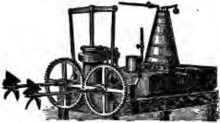
FIG. 84.—Engine, Boiler, and Screw-Propellers used by Stevens, 1804.
