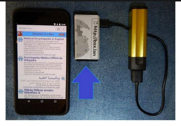
The Offline Distribution System for Medical Content is a mini computer that generates a wifi signal to which up to 32 people can connect at any one time with a computer or phone to access the content on the device. It also functions as a mini app store in that you can developed and install offline Wikipedia medical appears
