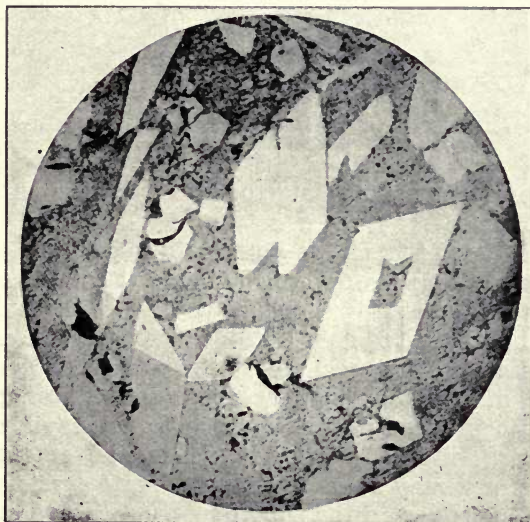
FIG. 37.—INGOT CONTAINING 10·17 PER CENT. PHOSPHORUS AND 88·9 PER CENT. IRON, SHOWING SECTIONS OF RHOMBIC OR OBLIQUE IDIOMORPHIC CRYSTALS OF Fe_3P EMBEDDED IN A GROUND MASS OF EUTECTIC. V \times 60 (STEAD).
