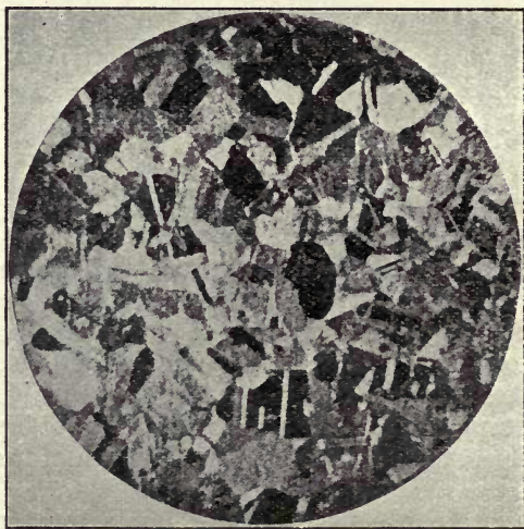
FIG. 41.—BRASS AFTER HEATING TO 600° C. (MAGNIFICATION 58 DIAMETERS.)
