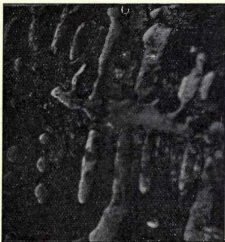
FIG. 93. Copper-lead alloy. Lead 25 per cent. V \times 230 .
