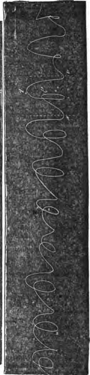
Fig. 30. Line 1. Chronographic trace of a tuning-fork, vibrating 100 times a second; 2. Vertical oscillations of the wild duck during flight. 3. Oscillations of the hen-hawk. 4. Of the screech-owl; and 5, of the harrier.
