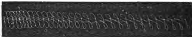
Trace of a Wheatstone's octave rod.
