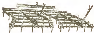
2331. Two types of tools for preparing the surface soil. The spike-tooth and spring-tooth harrows.
