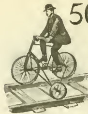
RAILWAY "SAFETY." WEIGHS ONLY 53 POUNDS. BALL BEARINGS AND MADE THROUGHOUT SIMILAR TO ROAD BICYCLE. FURNISHED WITH RUBBER CUSHIONED TIRES.
