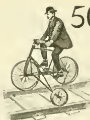
RAILWAY "SAFETY." WEIGHT ONLY 53 POUNDS. BALL BEARINGS AND MADE THROUGHOUT SIMILAR TO ROAD BICYCLE. FURNISHED WITH RUBBER CUSHIONED TIRES.
