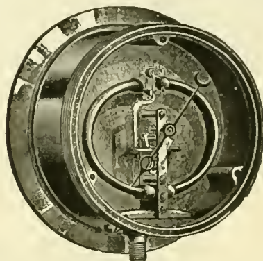
Movement no connection to back of case.
