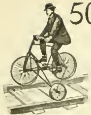
RAILWAY "SAFETY." WEIGHT ONLY 53 POUNDS. BALL BEARINGS AND MADE THROUGHOUT SIMILAR TO ROAD BICYCLE. FURNISHED WITH RUBBER CUSHIONED TIRES.
