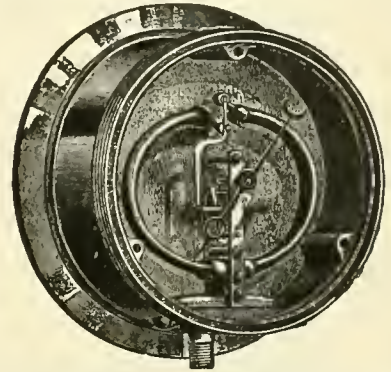
Movement no connection to back of case.
