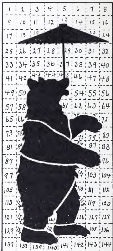
Plate 16.—Pantagraph, Used in Enlarging or Reducing Stencil Designs; Also the Square Method.
