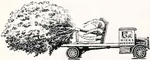
Tree-Mover No. 21. Moves evergreens and other trees with very large balls of earth. This is one of two Pines moved from our nursery to the church half a mile east. The big steel platform and frame are worth seeing
