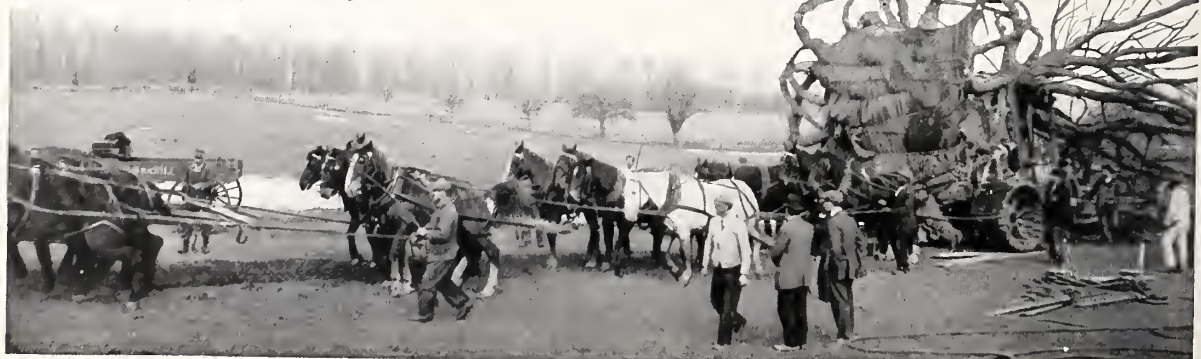
Tree-Mover No. 20. Moving large tree with a spread of roots of 50 feet. The wheels are 30 inches wide and both front and rear wheels are on pivots. The steel construction enables it to carry trees 33 inches in diameter with a large ball of earth in the center. Some trees have been 84 feet high and others 75 feet wide.
