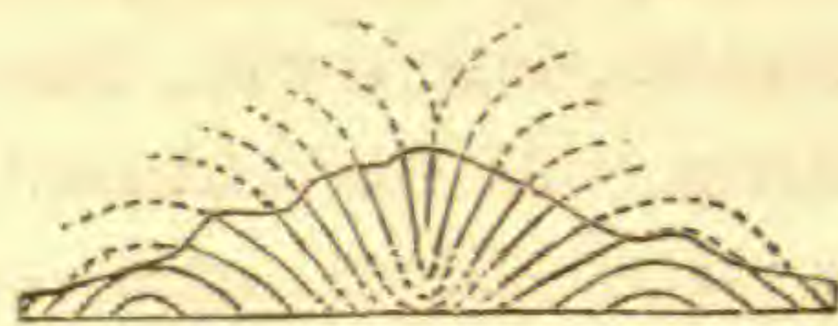
Ideal section showing how fan-structure may be produced by erosion of a syncline.
