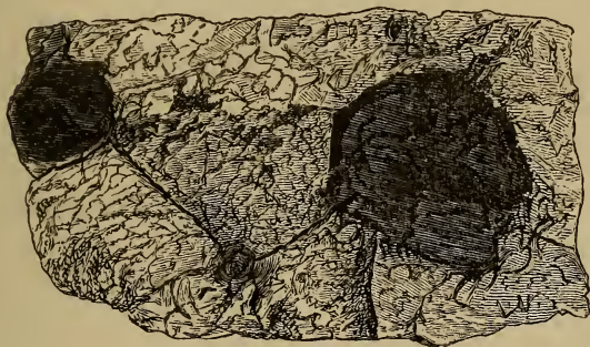
Fig. 7.—Top view of Mica-schist, showing flattened Garnets.
