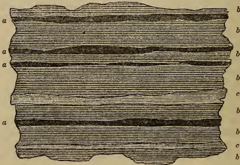
Fig. 1.— Diagram illustrating the Structure of the South-African Coals.
