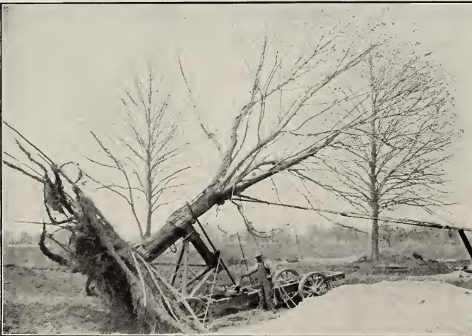
One of the Hicks' Patent Tree-Movers. —We have invented the method of digging which preserves the small feeding roots. The roots have a spread of 30 or 40 feet. After digging, the tree is grasped by the hinged cradle and swung over horizontally by a screw. In this position trees may pass under electric wires.
