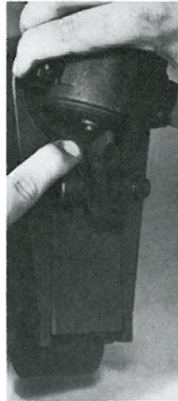
DEPRESS LOCKING PIN . . . ROTATE TO UNLOCK AND REMOVE BACK PLATE ASSEMBLY
