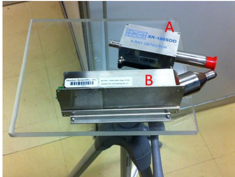
Figure 3 – Photograph of the portable ED-XRF system: A) Detector; B) X-ray tube with silver anode (Amptek®). Photo by the authors.
