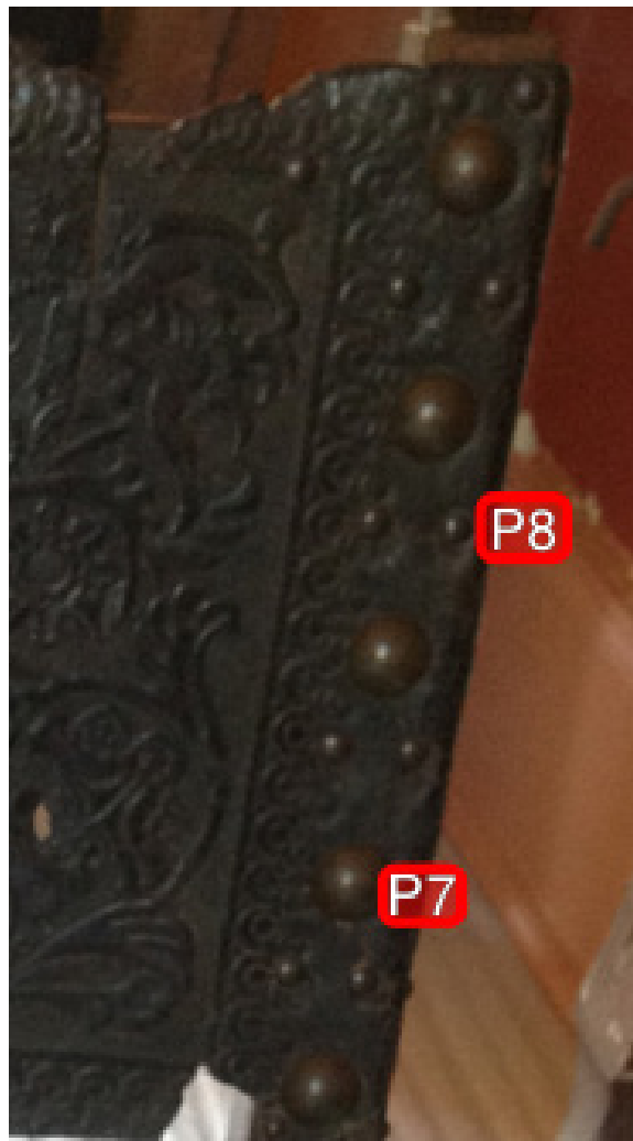
Figure 11 – Detail of the incidence of measurements in points P7 and P8, large and small upholstery nails, respectively, of the piece RG55 chair, belonging to the Museu Paulista collection. Photo by the authors.
