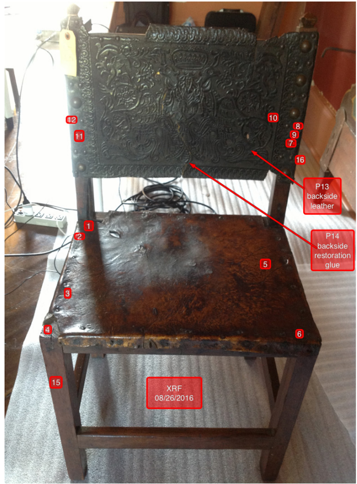
Figure 9 – Picture of visible light of the RG55 chair of the Museu Paulista collection with the identification of the different points measured by ED-XRF. Photo by the authors.
