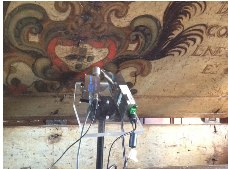
Figure 3 – Photograph of the portable ED-XRF system: A) Detector; B) X-ray tube with silver anode (Amptek®). Photo by the authors.
