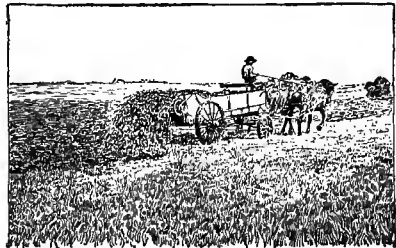
FIG. 65. Spreading manure with a manure spreader. This manure was pitched from the stable to the spreader—handled once only. (See Fig. 63.)
