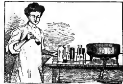
FIG. 177. Mixing milk and acid. A rotary motion with the bottle not pointed toward the face.
