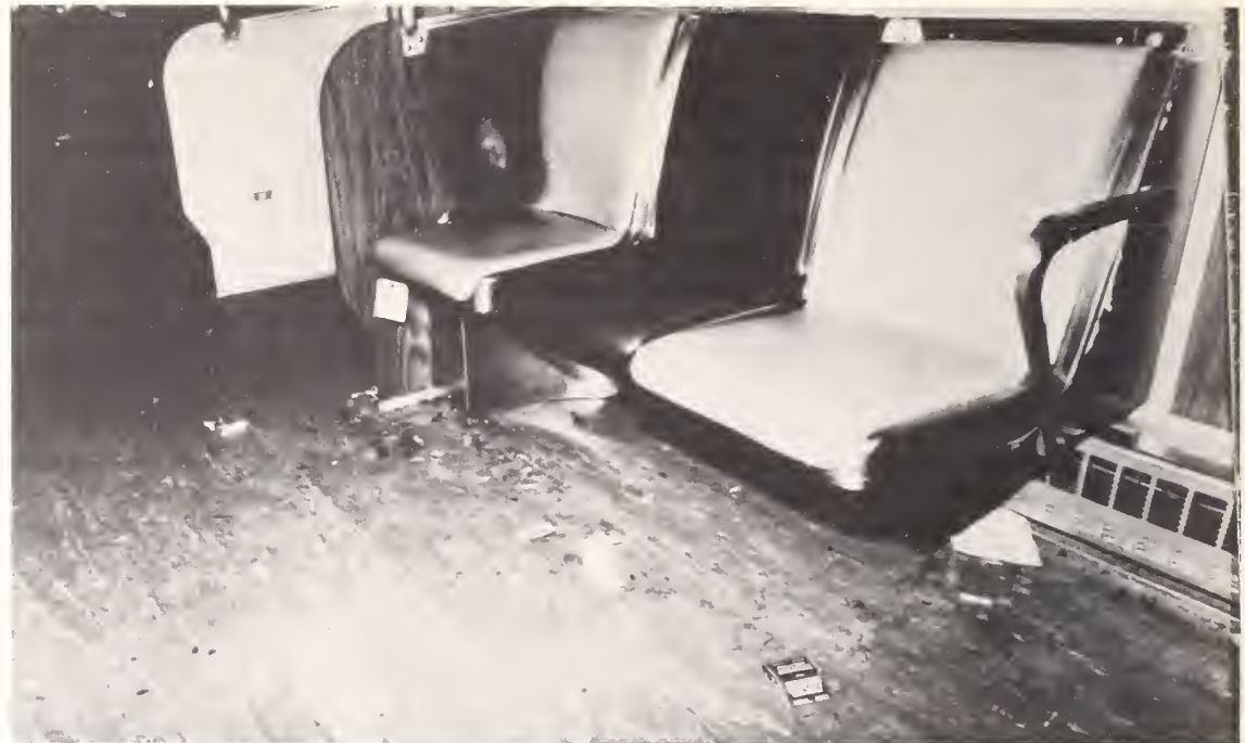
Use of fire-retardant materials prevented the spread of fire in this incident of attempted arson in a subway car.
