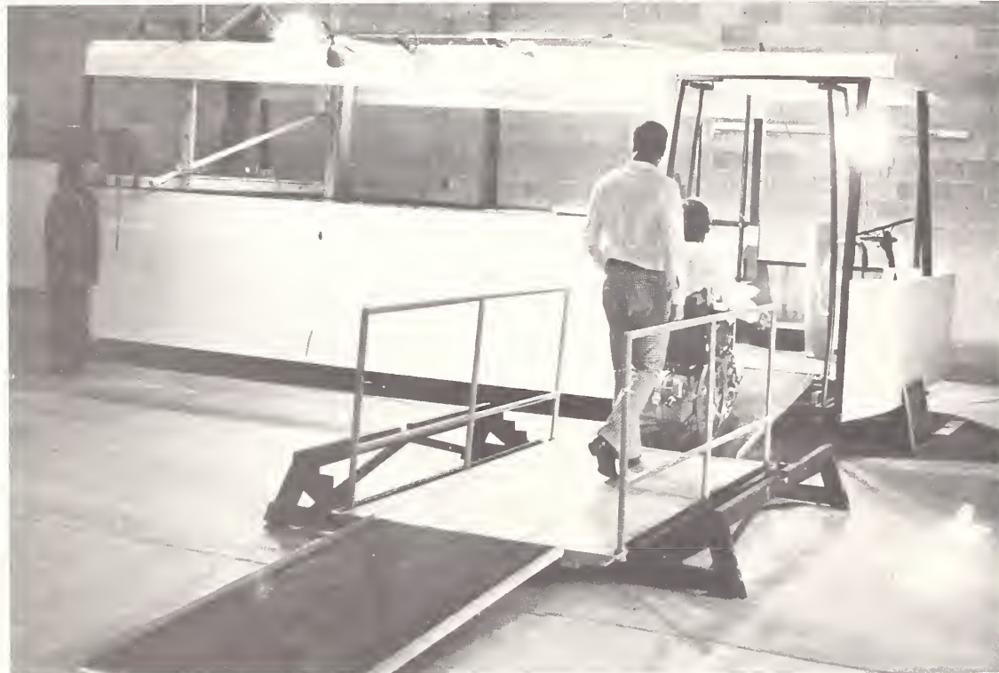
Tests are being conducted on the Transbus ramp mock-up with a simulated curb and a six-inch grade.
