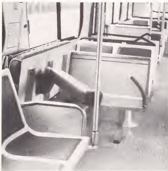
The jolts of normal traffic can be dangerous as well as uncomfortable for wheelchair users. Shown here is one method for securing wheelchairs. A curved spring snaps over the rear left wheel and a padded bar protects the passenger.
