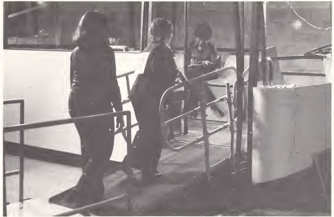
Another ramp design for Transbus features a 35-inch high handrail.
