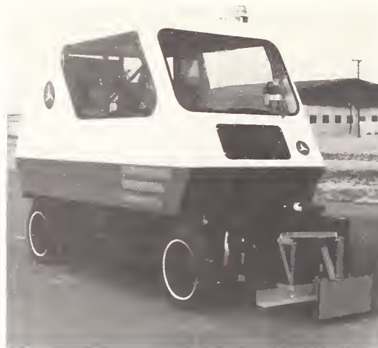
This research vehicle receives lateral control signals from a wire imbedded in the road.
