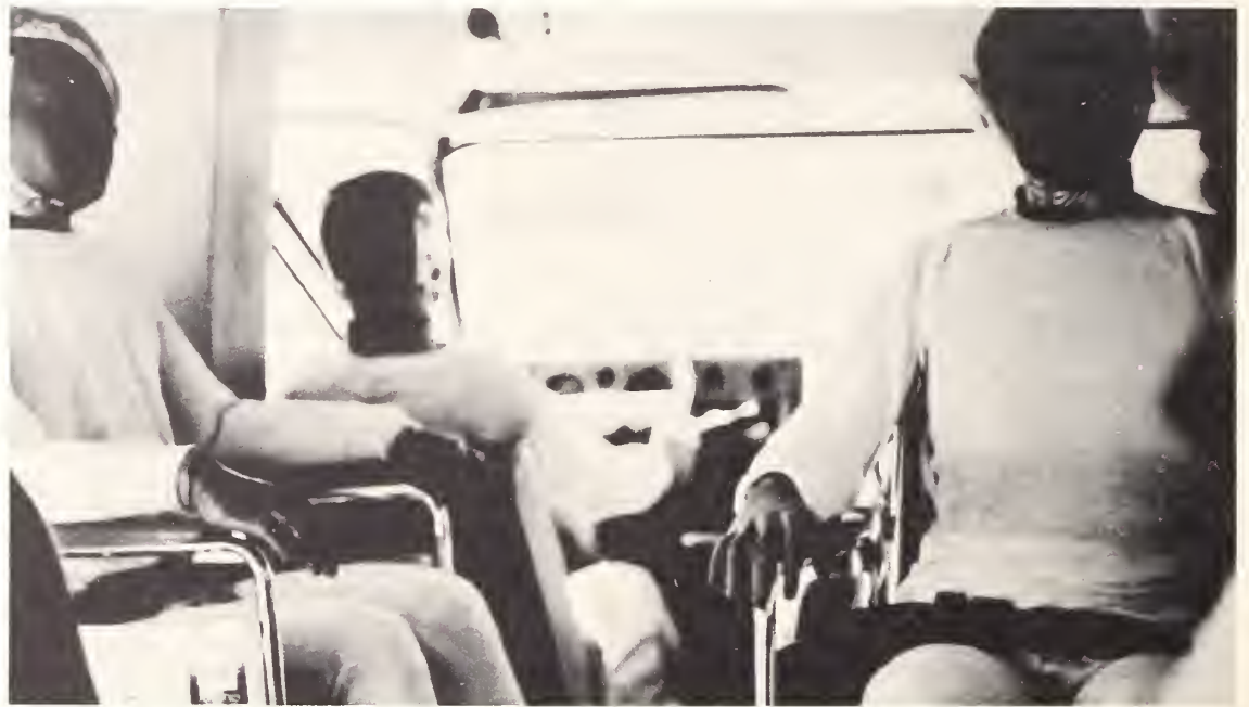
Crash protection systems for wheelchair occupants are being tested jointly with the National Highway Safety Administration's schoolbus test program.
