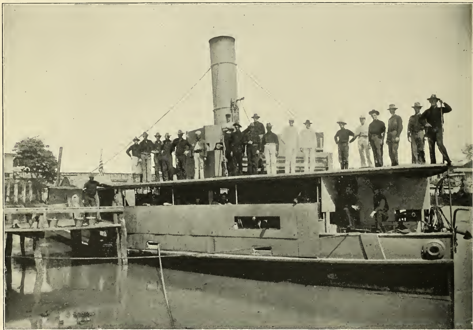
Gunboat Laguna de Bay —At the outbreak of hostilities this government was prepared to dislodge the insurgents from their strongholds along the Pasig and lake regions with the fleet of "tinclads," of which the above was the most formidable. Carrying two three-inch guns forward, two Nordenfeldts at the stern and four Gatlings above, she poured a deadly fire that quickly routed the enemy.
