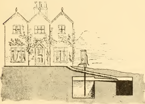
Fig. 593. New Vicarage Cesspool overflowing into a Tank.
