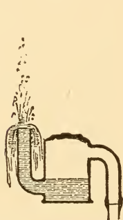
Fig. 276. Effect of Back Pressure.
