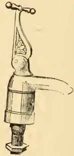
Figs. 369 and 369a. Section and Perspective iew of the Writer's Slow Closing Faucet.
