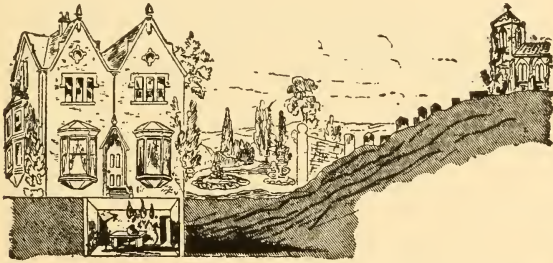
Fig. 636. Vicarage rendered unhealthy by infiltration from churchyard.
