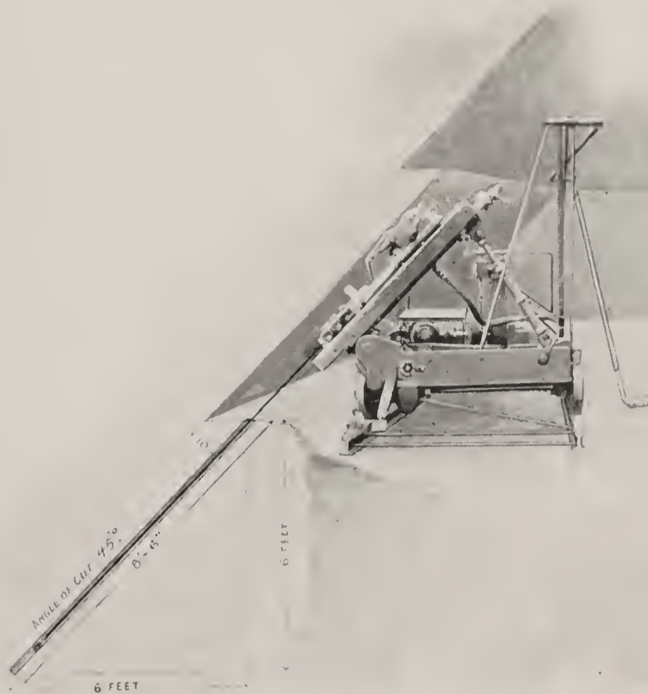
Fig. 69. Size No. 6½, Without Boiler. Making an Angle Wall Cut.
