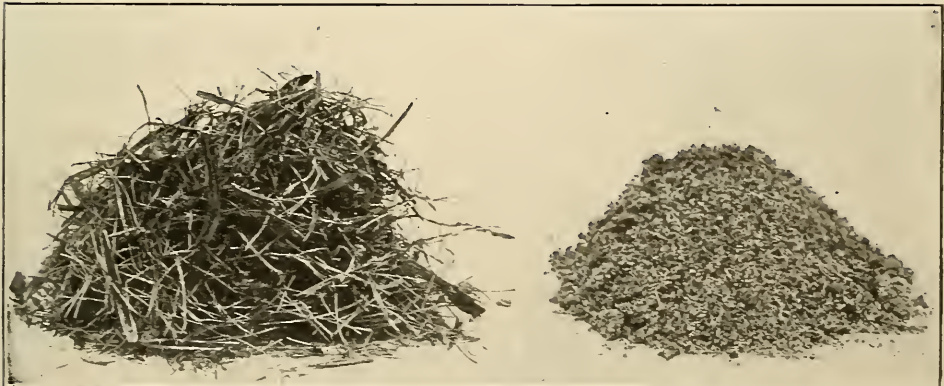
The cane and pith of the sugar stalks, after it has passed through the defibering and drying process of the plant at Preston, Nipe Bay. A view of the factory will be found on the preceding page.
