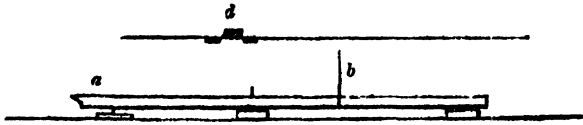
a, Key. b, Brass pin wire. c, String. d, Cloth woven between the strings as a damper.
