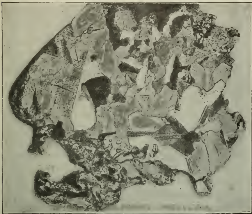
ETCHED SECTION OF SAME NUGGET, SHOWING CRYSTALS.
