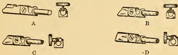
Fig. 10.—Compass Leg Joints.
