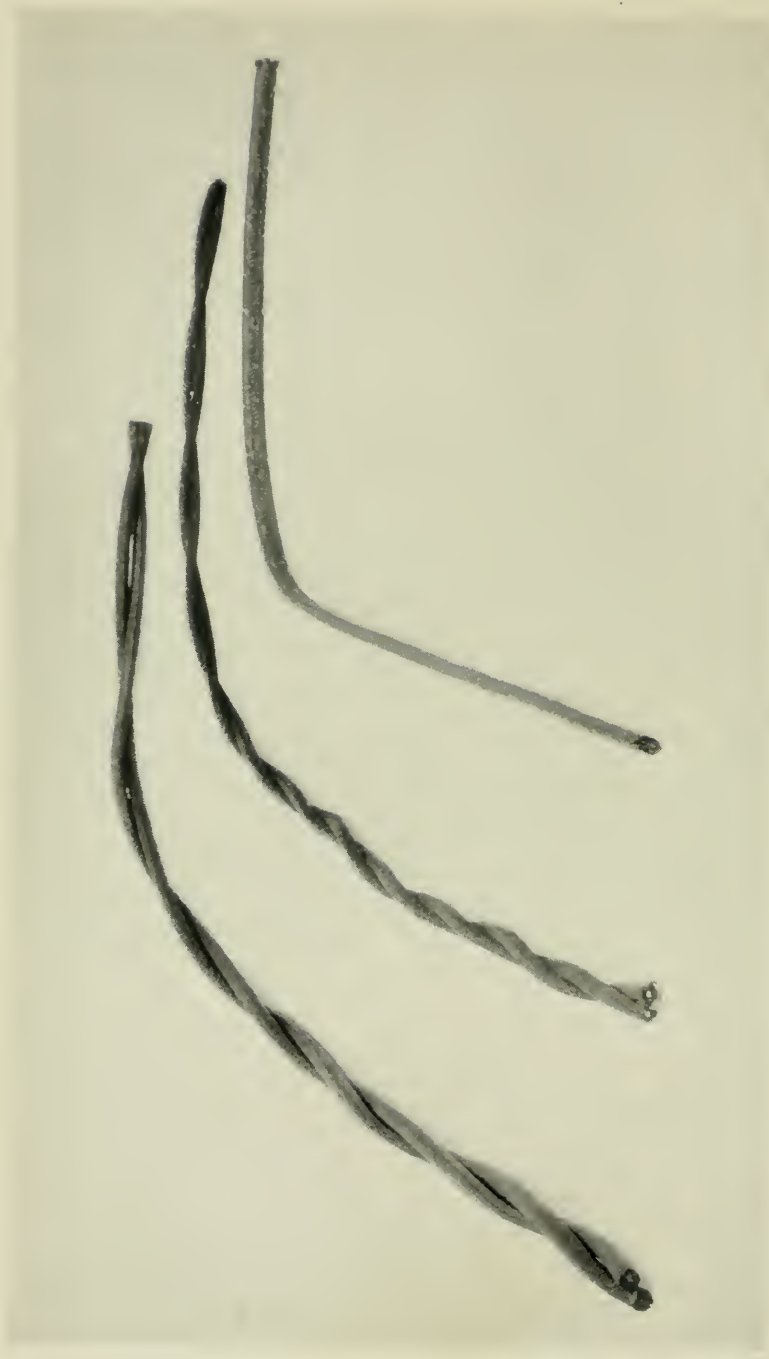
FIGURE 2. THREE STAGES IN THE DEVELOPMENT OF DROP WIRE USED IN THE BELL SYSTEM.
