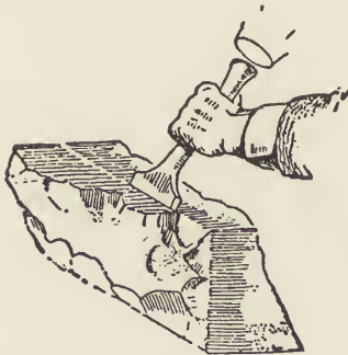
Fig. 77.—Rock-face or Pitch-face.
