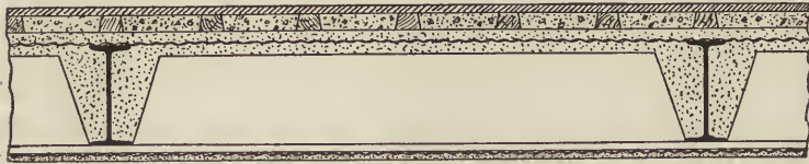
No. 3.—Span, 6 feet ; weight, 35 lbs. per sq. foot.
