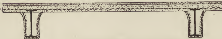
No. 5.—Span, about 8 feet ; weight, 30 lbs. per sq. foot.
