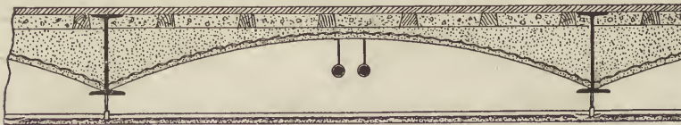
No. 9.—Span, 6 feet ; weight, 45 lbs. per sq. foot.
