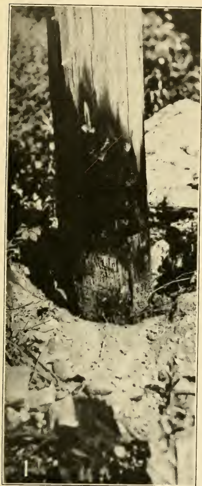
FIG. 1.—Chestnut telephone pole, with base charred but basal area untreated. This pole has been standing near Dover, N. J., for eight years. (Photograph loaned by United States Forest Service.)
