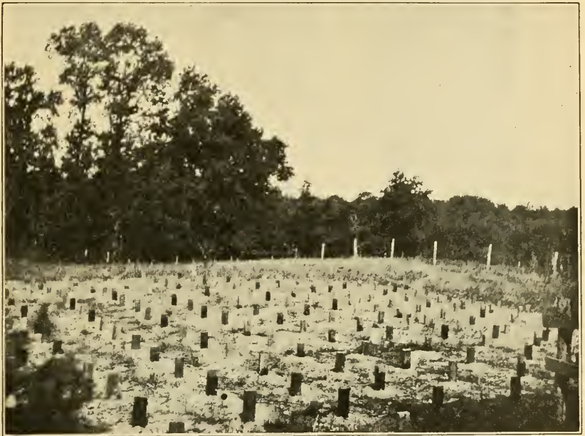
FIG. 4.—View at Falls Church, Va., showing a portion of the treated experimental stakes under test, as to the relative effectiveness of preventives against termite attack. (Original.)
