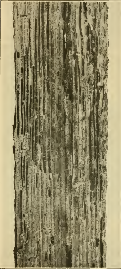
FIG. 6.—Work of termites in insect-killed southern yellow pine. Tree killed in the spring; wood at base honeycombed by following December. Spartanburg, S. C. (Original.)
