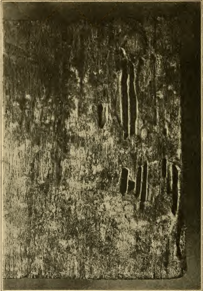
FIG. 14.—Red oak block, impregnated with paraffin wax, honeycombed by termites after five months' test. This was buried in the ground with termite-infested logs. (Original.)
