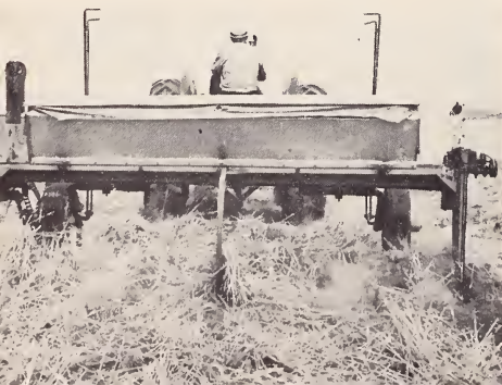
New-type drill designed and built by an ingenious farmer for the purpose of placing seed in the ground beneath heavy trash cover. This machine is still in experimental stage.
