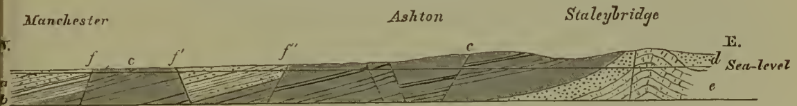
FIG. 43. Section across the Manchester Coal-field from West to East. (After the Geol. Survey.) (Horizontal and vertical scale \frac{1}{4} inch = 4000 feet.)
