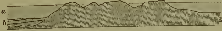
FIG. 6. Ideal Section through Charnwood Forest. a New Red Sandstone; b Coal-Measures; x Cambrian or Pre-Cambrian Rocks.
