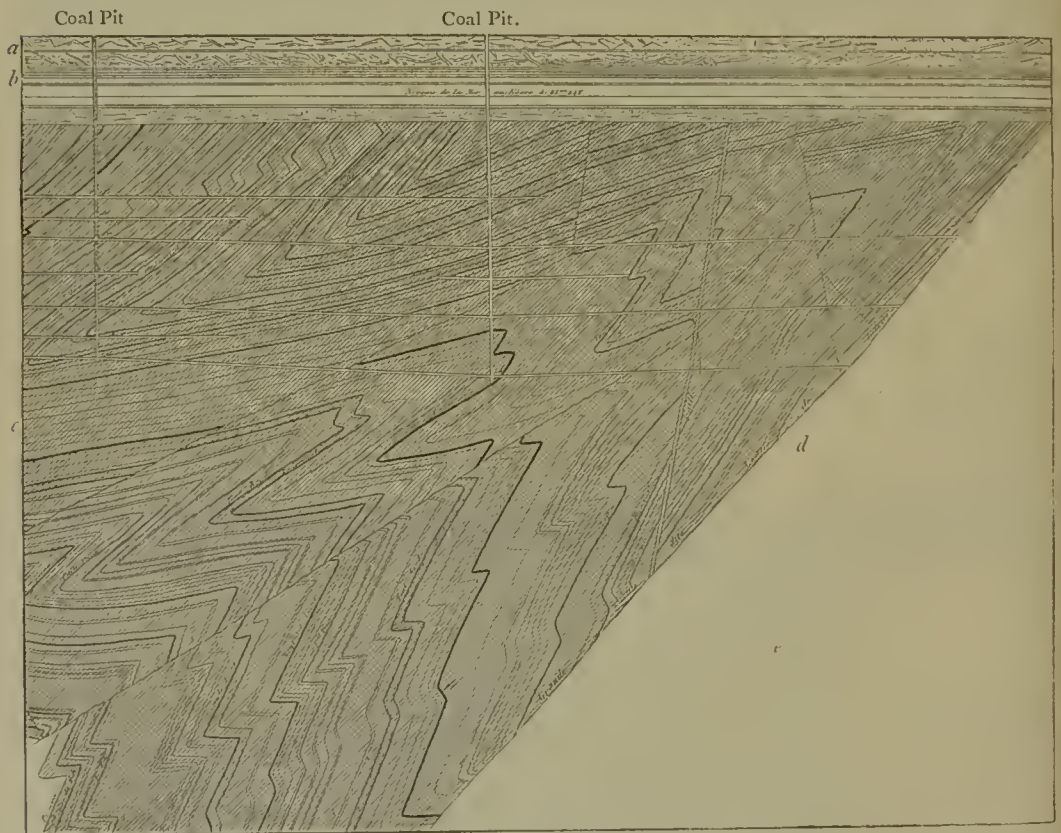
FIG. 44. Diagram Section in the Collieries of St. Vaast Anzin; Coalfield 'Du Nord.' (After Burat ) a. Lower Tertiary Strata, and b. Chalk (300 to 400 feet). c. Coal-measures. d. Great Fault. e. Broken Ground.
