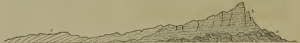
FIG. 4. Generalised Section of the Cambrian conglomerates (b) resting on Laurentian Gneiss (a) in western Ross-shire and Sutherland (Murchison). (c) Silurian Strata.
