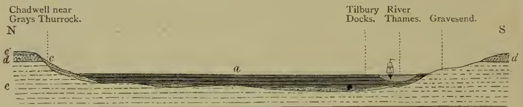
FIG. 253. Section across the Thames Valley at Tilbury. a. Alluvial Beds. c. Low-level Drift. e. High-level Gravel. d. Lower-Tertiary Strata. e. Chalk.
