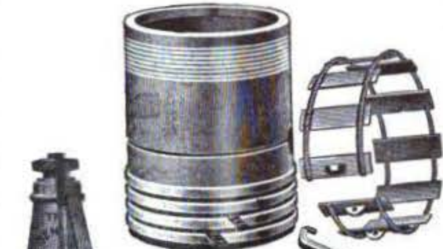
The Morgan piston ring compressor.
