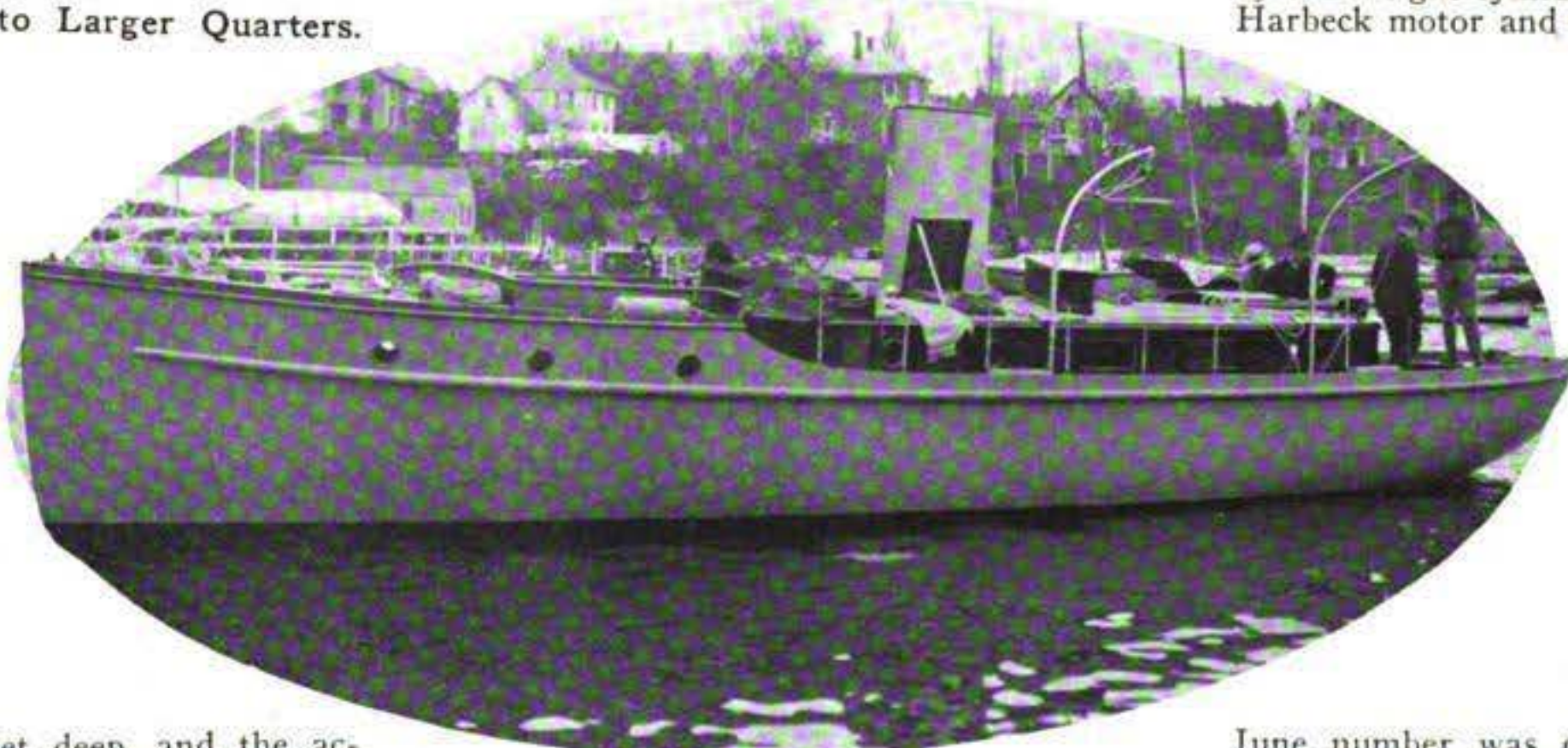
Putting the finishing touches on Alsortie III, a cruiser built by the Camden Anchor-Rockland Machine Co., of Camden, Me., for C. N. Burnell, of Boston, Mass. She measures 51 feet length by a beam of 10 feet 1 inch.
