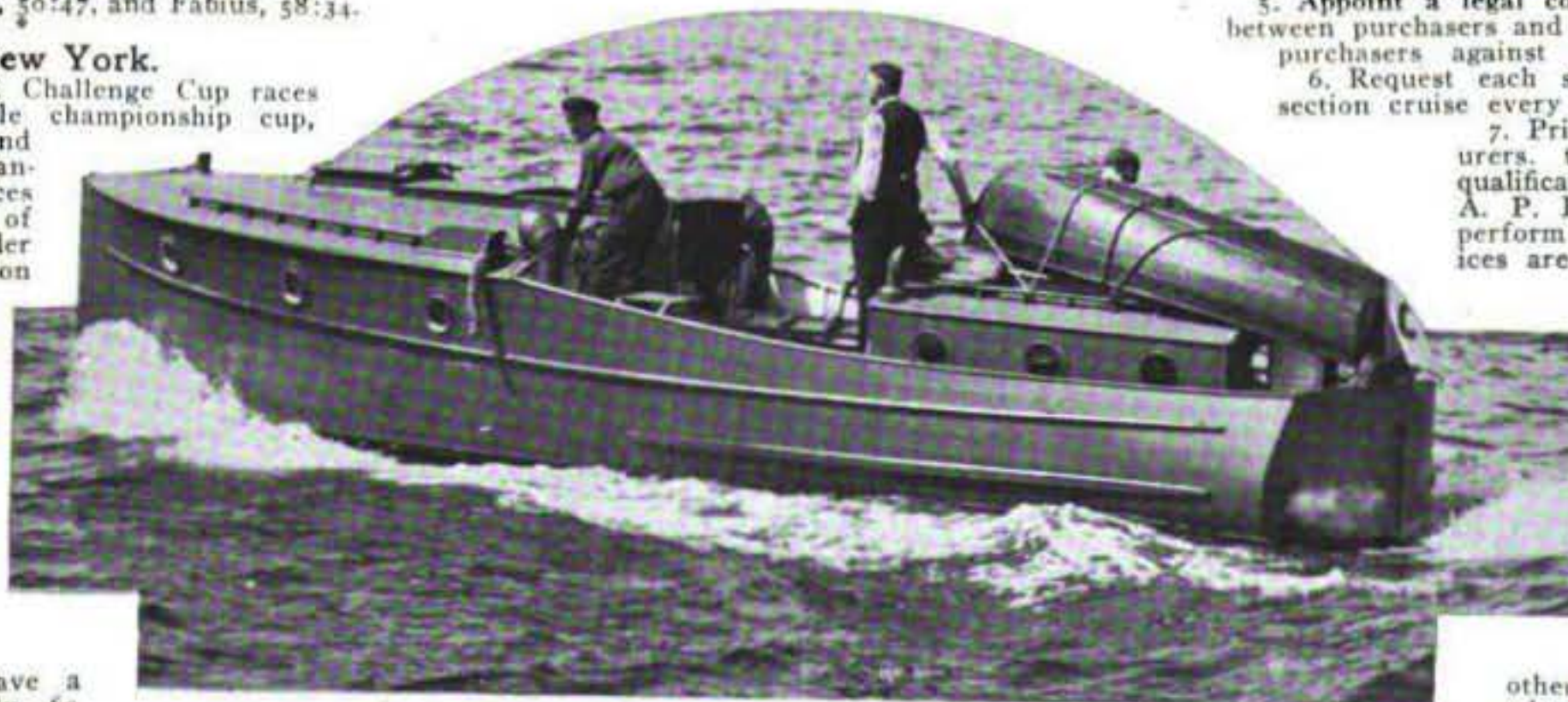
Katy Did, the new Hand V-bottom cruiser owned by J. K. Van Denberg, of the Colonial Yacht Club, and powered with a four-cylinder, 5 1/2 x 6 3/4-inch Sterling motor.
