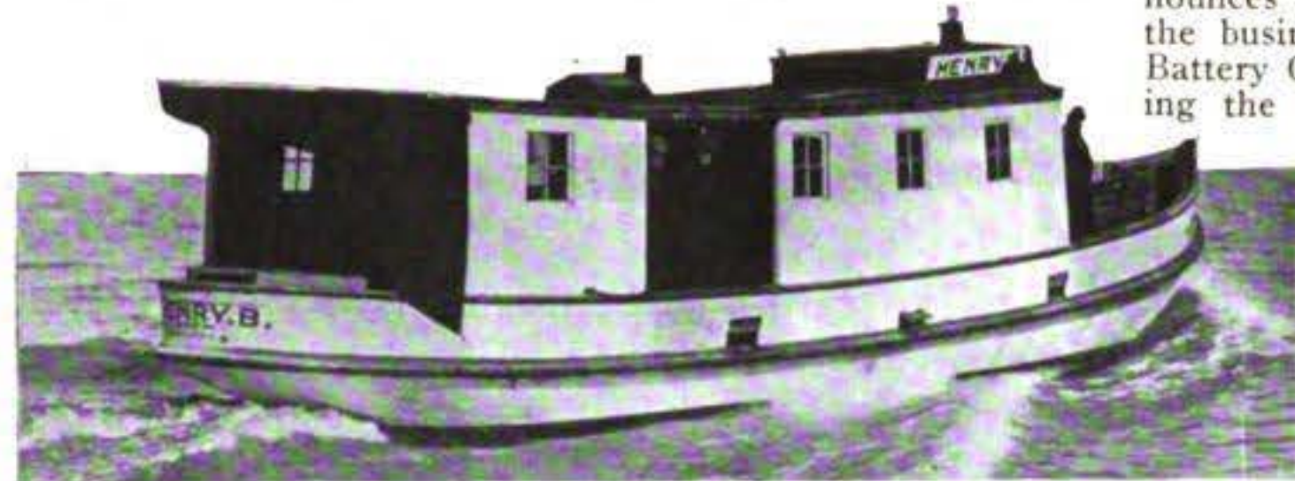
Henry B. a Great Lakes commercial motor boat which is powered with a heavy-duty Sterling and makes her 12 miles right along.
