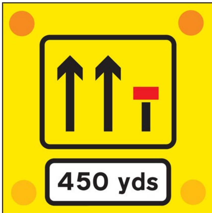
Signs used on the back of slow-moving or stationary vehicles warning of a lane closed ahead by a works vehicle. There are no cones on the road.
