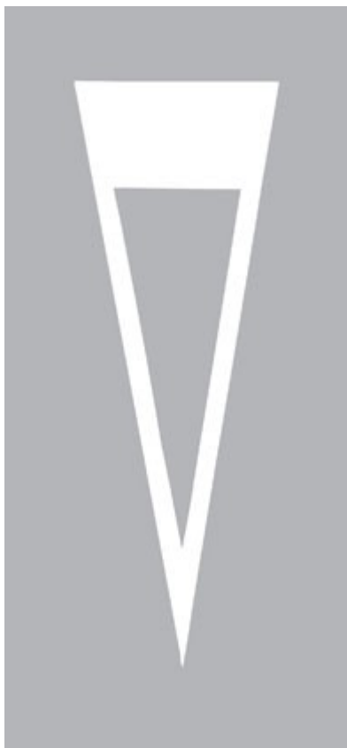
Warning of 'Give Way' just ahead
