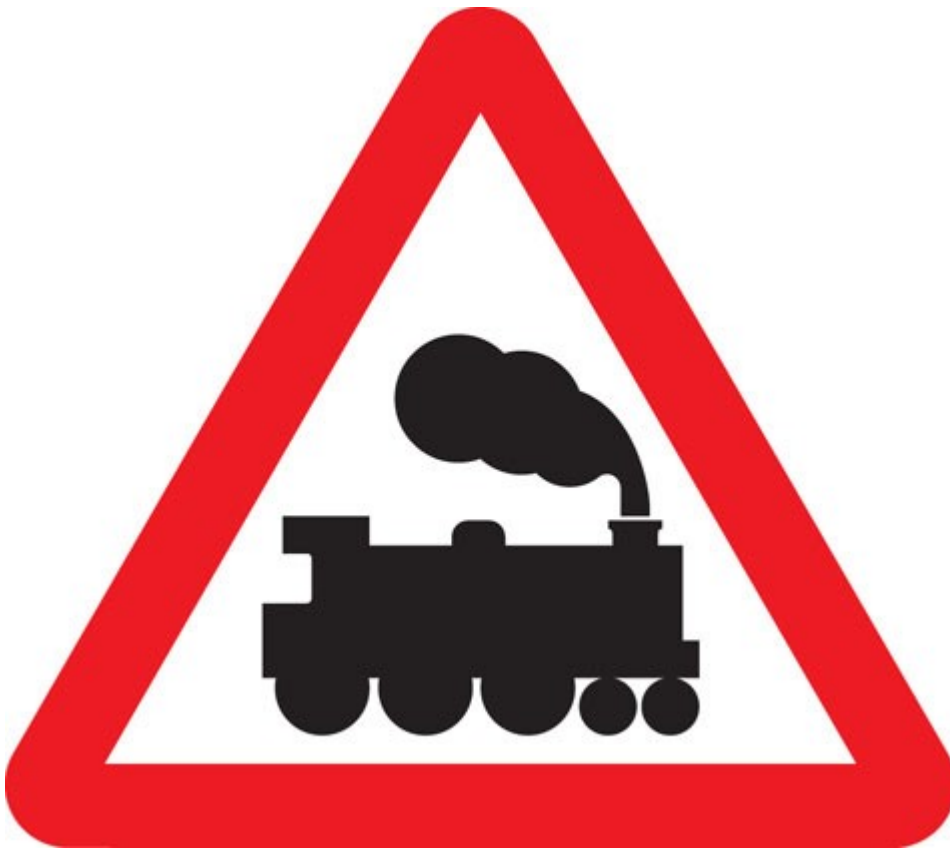
Level crossing without barrier or gate ahead
