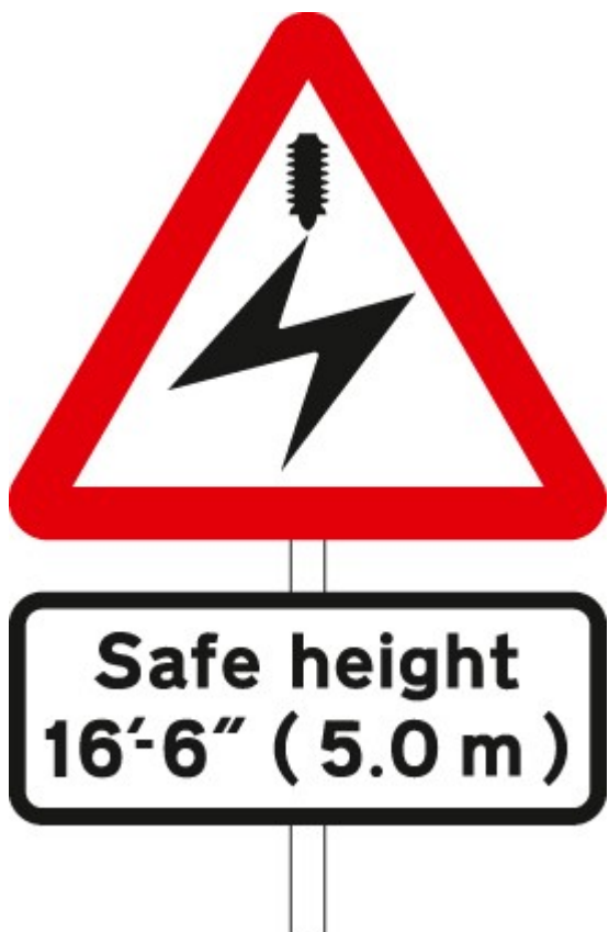
Overhead electric cable; plate indicates maximum height of vehicles which can pass safely
