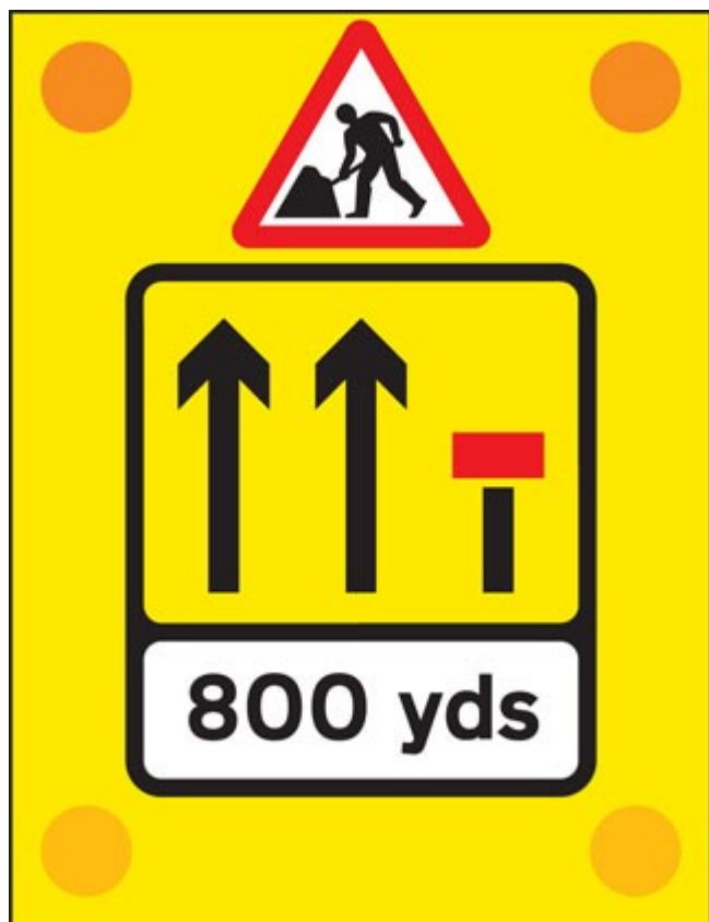
Signs used on the back of slow-moving or stationary vehicles warning of a lane closed ahead by a works vehicle. There are no cones on the road.
