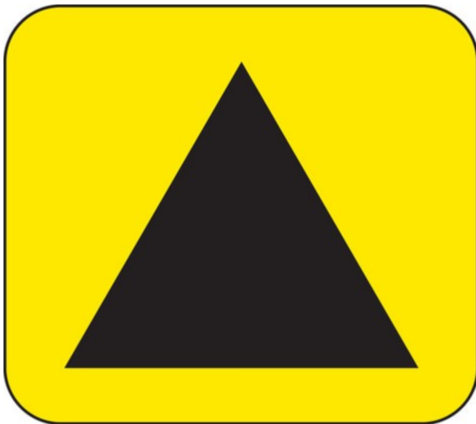
Symbols showing emergency diversion route for motorway and other main road traffic
