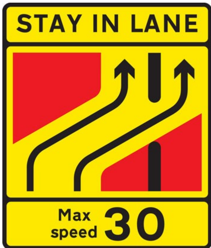
One lane crossover at contraflow road works
