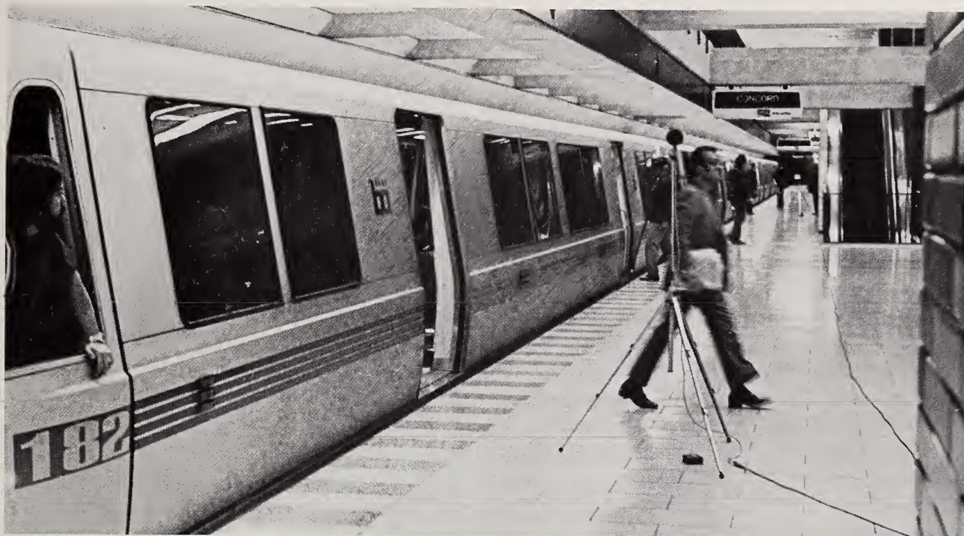
Microphones placed in stations measure sounds of arriving and departing trains as part of the assessment program.
