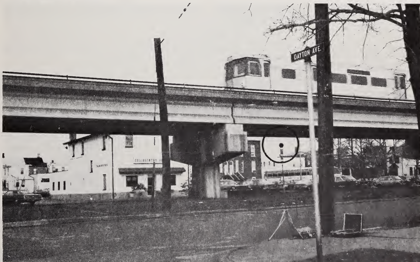
Noise levels of moving trains are measured at specified distances from the track on each of the nine transit systems studied.
