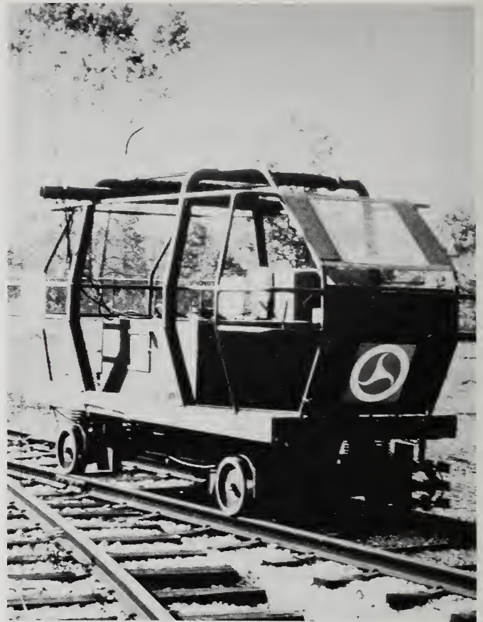
Experiments performed with this test vehicle were used to verify wheel/rail noise models.
