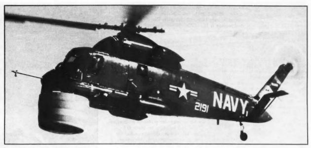
This Navy HH-20 Seasprite helicopter is equipped with a newly developed radar antenna system. The six-foot, eight-inch diameter radome, located under the nose, can be inflated to 52 inches in depth (as shown). The inflatable radome does not reduce the helicopter's landing ability.
