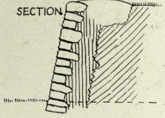
FIG. 164. -- DRY WALLING (SECTION). TIGHTLY RAMMED EARTH SHOWN BY VERTICAL HATCHING.
