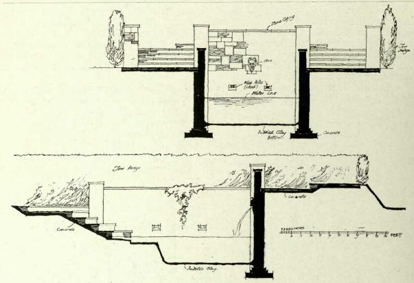
FIG.205. —CROSS AND LONGITUDINAL SECTIONS THROUGH LILY POND, MILLFIELD.
