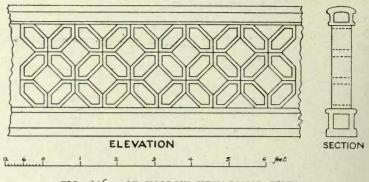
FIG. 136.—OF HOLLOW HEXAGONAL TILES.
