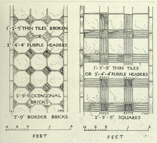
FIG. 251.—BRICK AND TILE PAVING.
