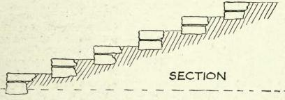
FIG. 165.—STEP WITH FRONT EDGES ONLY OF STONE.
