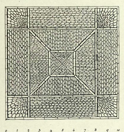
FIG. 240.—A SUMMER-HOUSE PAVING OF IRONSTONE AND BARGATE STONE.
