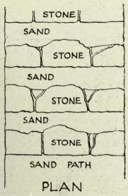
FIG. 163.—STEPS WITH FRONT EDGES ONLY OF STONE.
