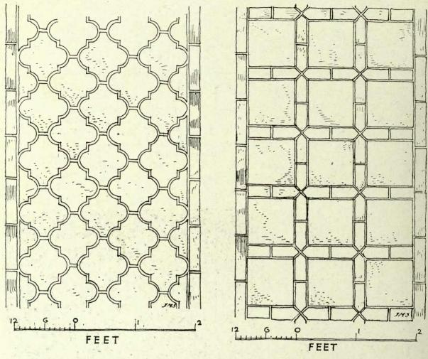
FIG. 253.—BRICK AND TILE PAVING.
