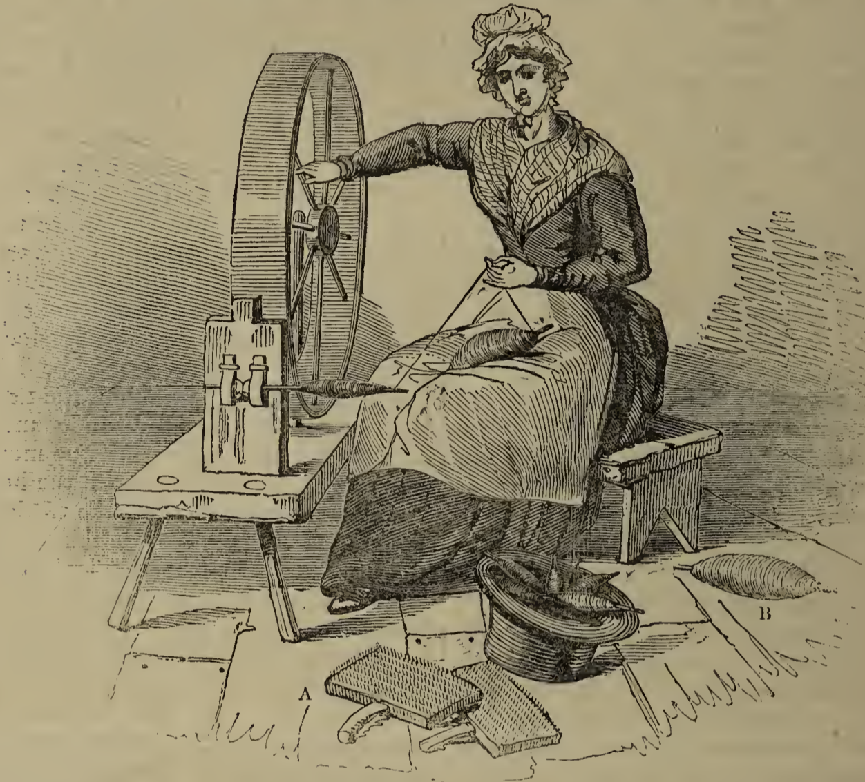
[The Jersey Wheel.—A and B are the hand-cards and bobbins of rovings.]
