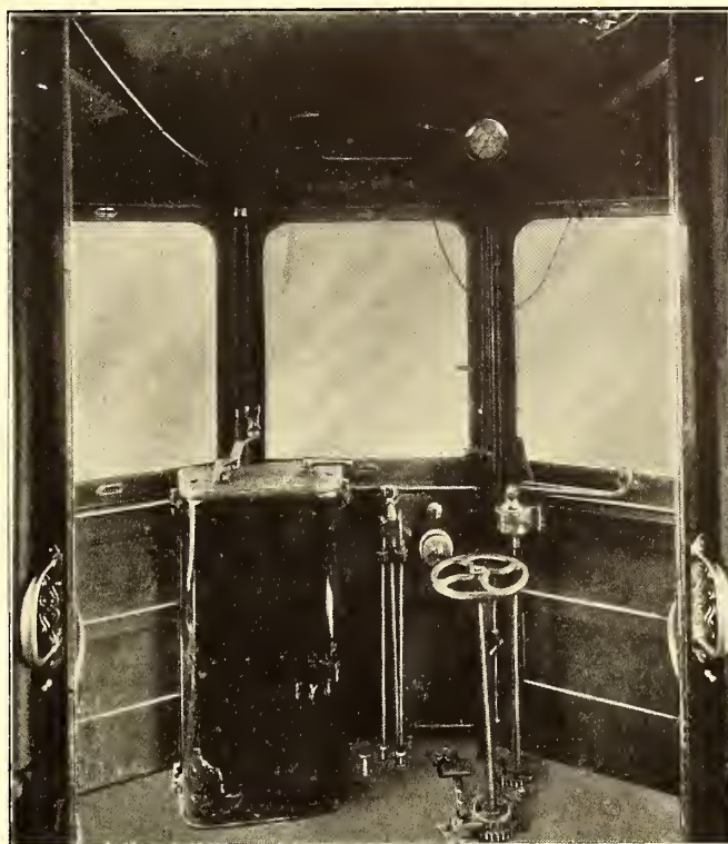
OPERATING PLATFORM OF INTERURBAN CAR WITH SINGLE-PHASE CONTROLLER
