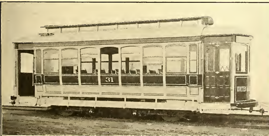
ONE OF THE NEW CONVERTIBLE CARS FOR CHATTANOOGA, SHOWING PANELS INSTALLED, BUT WITH PART OF THE WINDOWS RAISED
