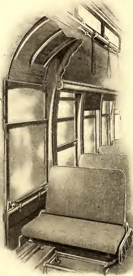
Brill Grooveless Post Semi-Convertible Car (Patented). Lower sash attached to upper by metal tongue-and-groove sliding connections. Rollers in brackets at top of upper sash move on bow-shaped steel guides and conduct sashes into roof pockets.
