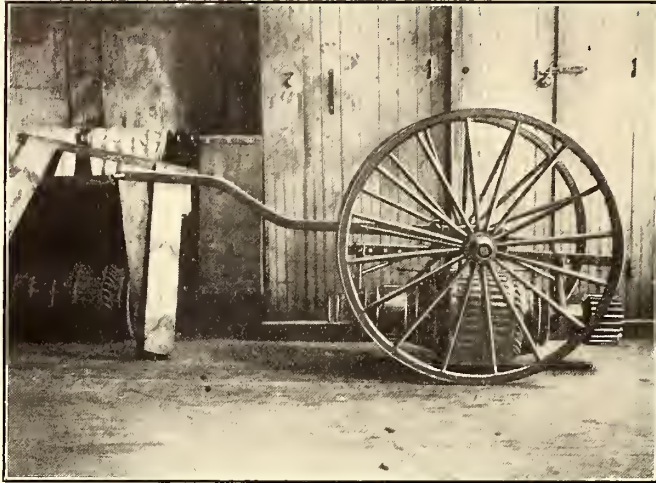
FIG. 5.—AN ARMATURE CART WHICH ELIMINATES HEAVY LIFTING
