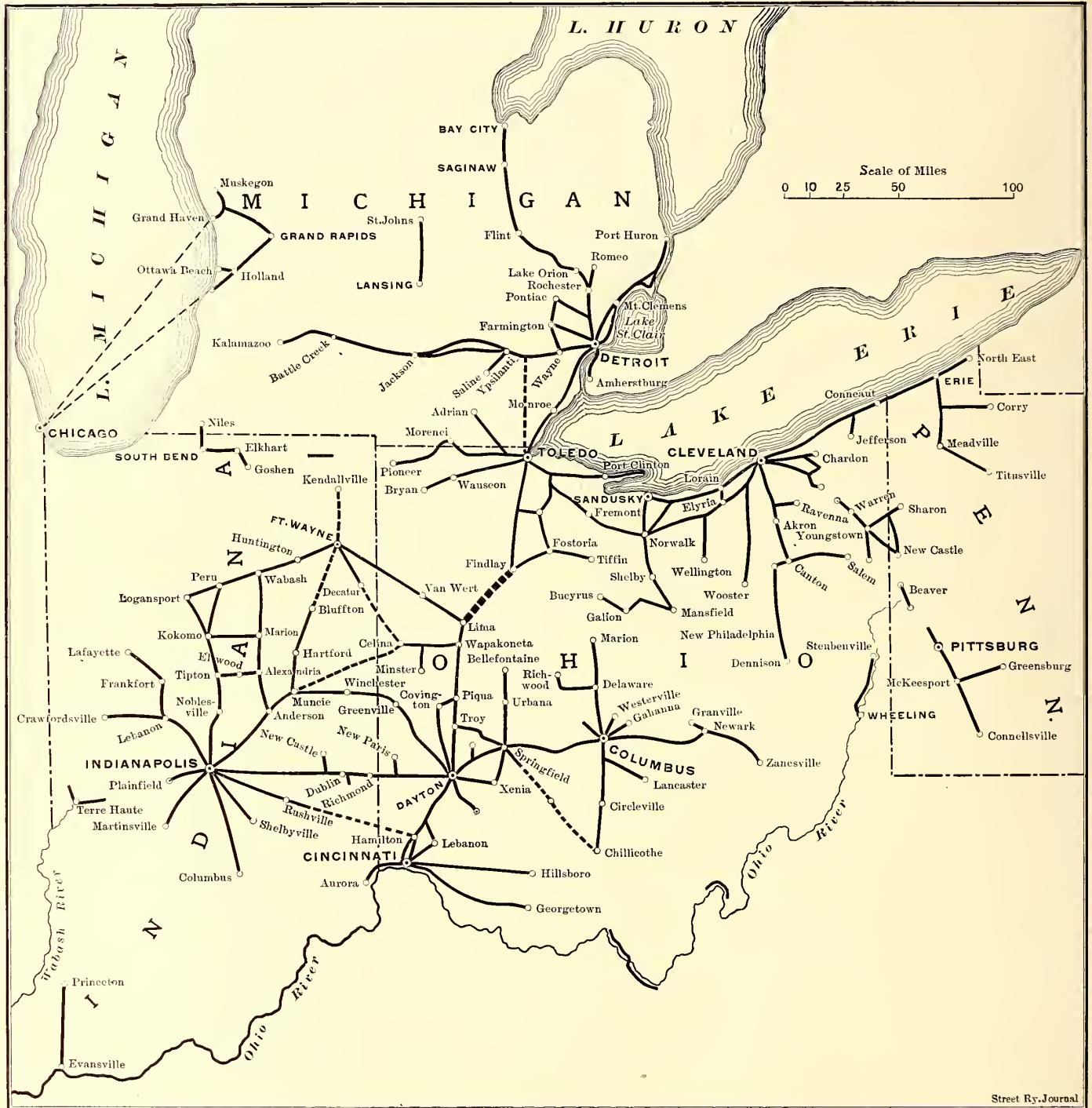
MAP SHOWING THE PRINCIPAL INTERURBAN ELECTRIC RAILWAY SYSTEMS IN OHIO, INDIANA, MICHIGAN AND WESTERN PENNSYLVANIA. THE CONNECTING LINK, WHICH WAS COMPLETED ON DEC. 30, IS INDICATED BY THE HEAVY DOTTED LINE BETWEEN FINDLAY AND LIMA. THE LIGHT DOTTED LINES SHOW PROPOSED LINES OR THOSE UNDER CONSTRUCTION
