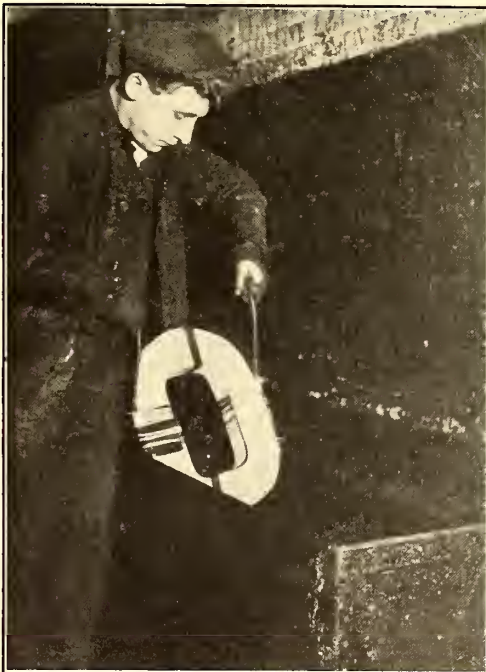
DIPPING FIELD COILS, MONTREAL STREET RAILWAY SHOPS
