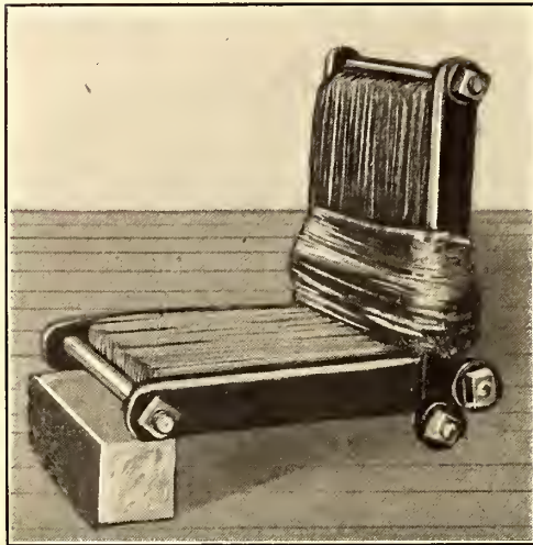
TRANSFORMER FOR TESTING ARMATURES, MONTREAL STREET RAILWAY SHOPS
