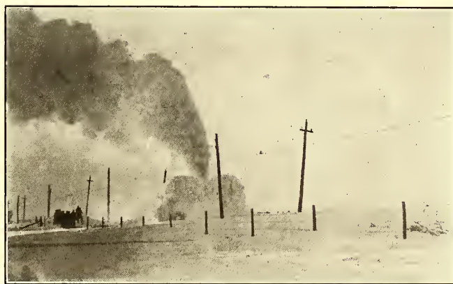
FIG. 2.—ENGINE STRIKING DRIFT HEAD ON
