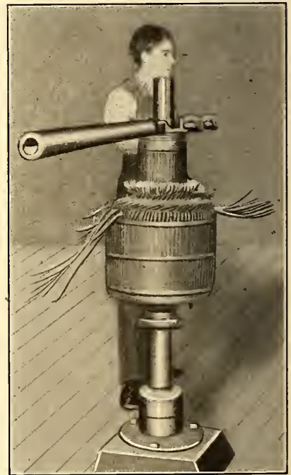
REMOVING COMMUTATOR COLLAR, MONTREAL STREET RAILWAY SHOPS
