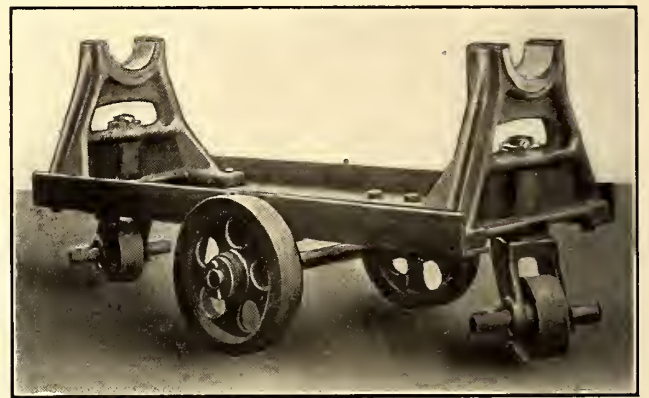
ARMATURE TRUCK WITH BABBITTED BEARINGS
