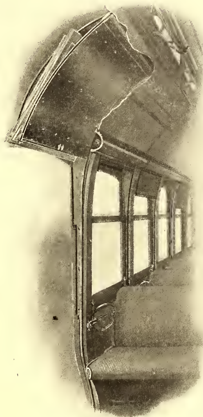
Section of Brill Grooveless Post Convertible Car (Patented). The Window System is the same as the Semi-Convertible. Flexible Metal Panels slide into Roof Pockets by means of metal guides on the posts.
