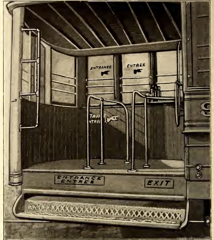
REAR PLATFORM OF "PAY-AS-YOU-ENTER" CAR, SHOWING EXIT AND ENTRANCE PASSAGeways
