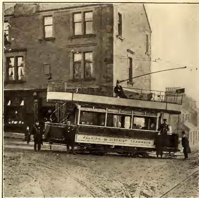
STANDARD DOUBLE-DECK CAR CLIMBING A GRADE ON THE LINE OF THE FALKIRK & DISTRICT TRAMWAYS
