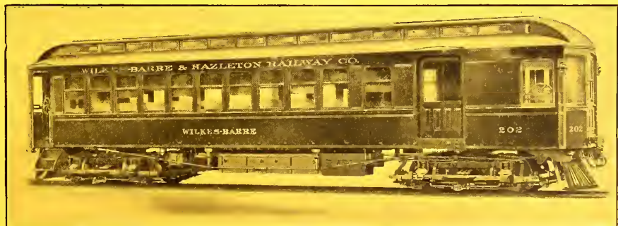
Combination passenger and baggage car for use on systems with conditions similar to steam roads. Length over body, 43-ft. Length over vestibules, 51 ft. Mounted on Brill No. 27-E-2 Trucks.
