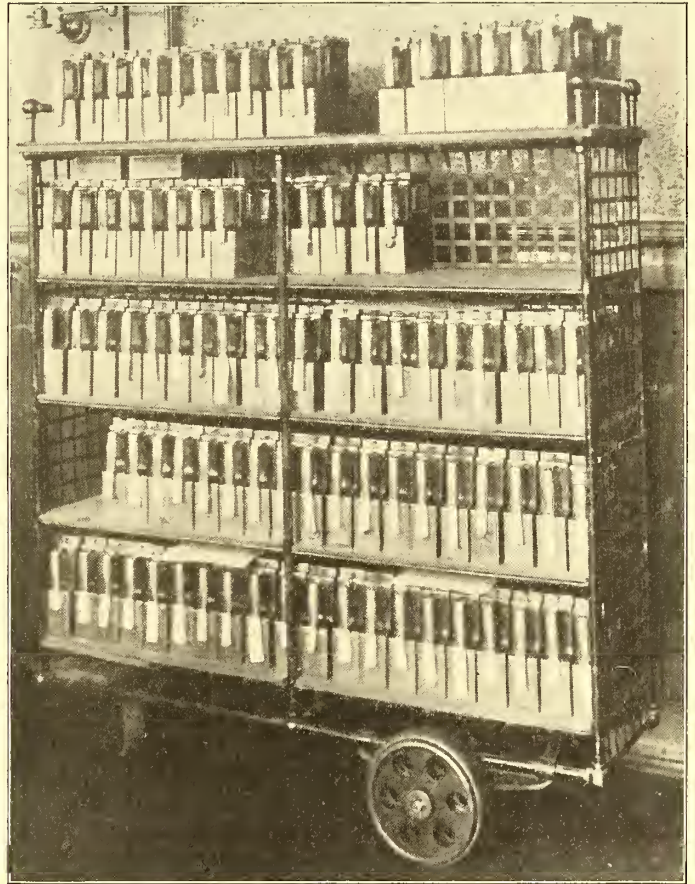
TRUCK USED FOR HANDLING FARE BOXES, TORONTO RAILWAY
