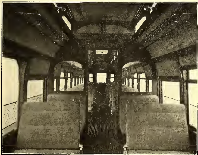
INTERIOR OF GULFPORT-BILOXI CAR, SHOWING DIVISION INTO COMPARTMENTS
