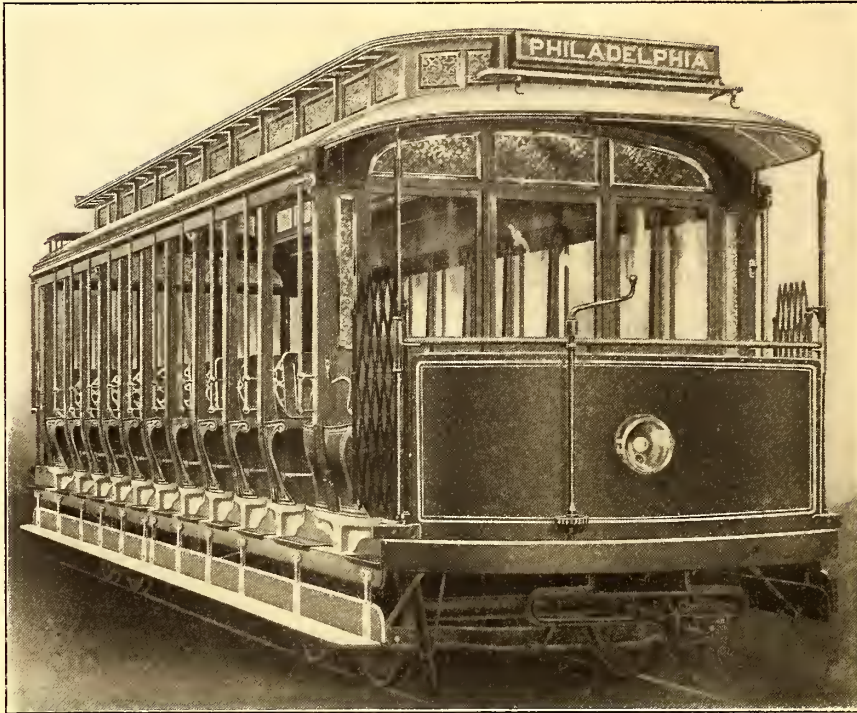
Brill Narragansett Car (Patented). No wider over all than a car without the sill step. Mounted on Brill No. 27-GE-1 Trucks.
