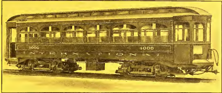
A type suited to systems which combine urban and interurban conditions. Length over body, 34-ft. Length over vestibules, 43-ft. 5-ins. Mounted on Brill No. 27-E-1½ Trucks.
