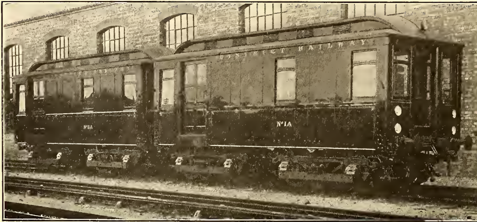
DISTRICT RAILWAY LOCOMOTIVE IN TWO UNITS
