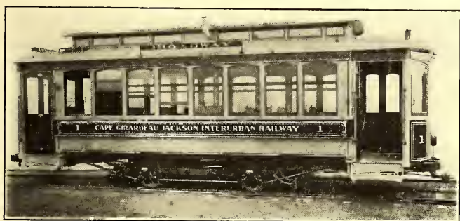
SINGLE-TRUCK CAR FOR THE CAPE GIRARDEAU & JACKSON INTERURBAN RAILWAY
