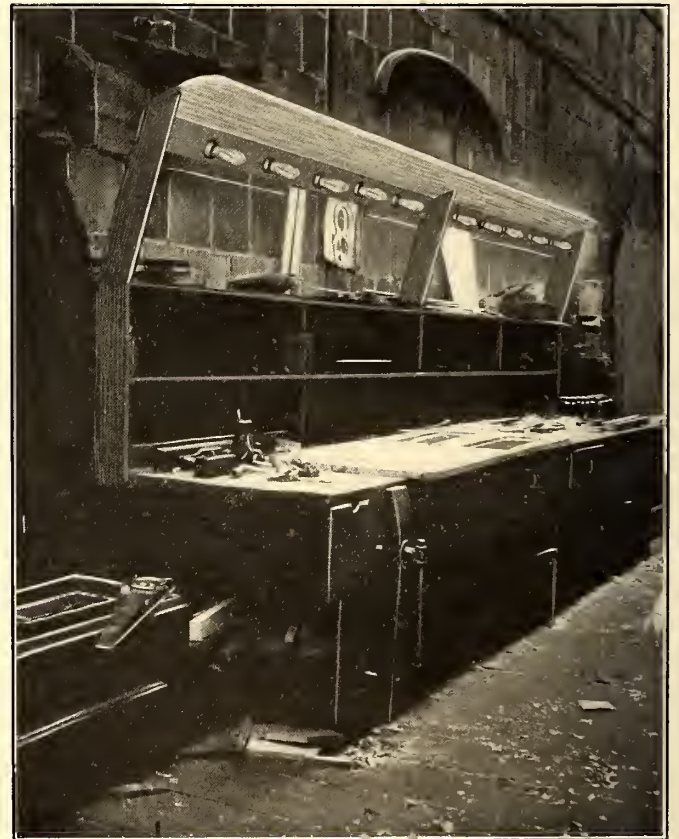
FIG. 2.—LIGHTING OF CARPENTER'S BENCH
