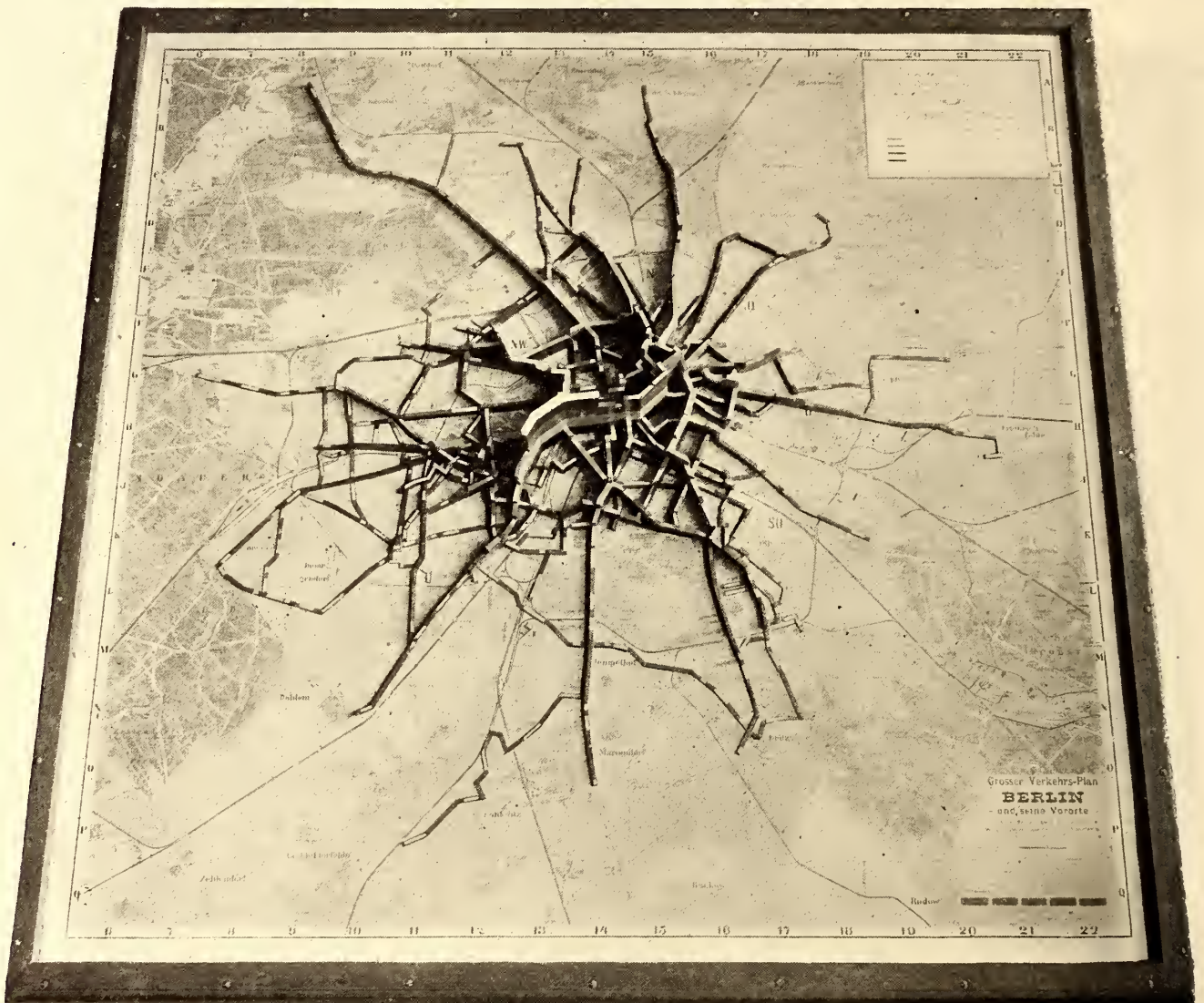
FIG. 3.—RELIEF MAP OF THE SURFACE RAILWAY SYSTEM OF BERLIN AND ENVIRONS, INDICATING THE DENSITY OF TRAFFIC
