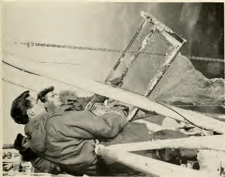
1. A trawl being prepared for lowering over the side of the ship. The mouth of the trawl is held open by the steel structure. A weight may be attached to the line in front of the trawl to keep it on the sea bottom. (Courtesy U.S. Navy Oceanographic Office.)
