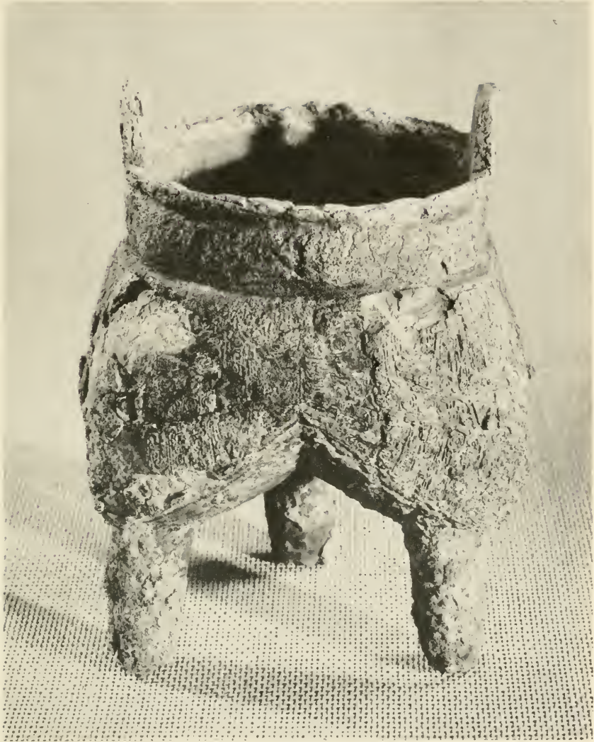
Chinese bronze ceremonial vessel of the type ting . Shang Dynasty. From long burial this ancient bronze has been almost completely altered to mineral products of copper, tin and lead, similar to the ore minerals from which those metals were originally derived. Courtesy: Royal Ontario Museum (Menzies Collection), Toronto.
