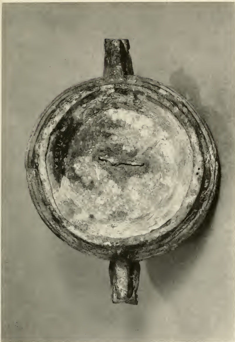
Chinese bronze ceremonial vessel of the type kuzi . Chou Dynasty. This view of the underside shows patches of whitish crystalline cerussite (lead carbonate) mixed with bright green malachite (basic copper carbonate). Lead was often added by early Chinese metallurgists to copper-tin melts used in casting vessels of this kind. Freer Gallery of Art (No. 11.58).
