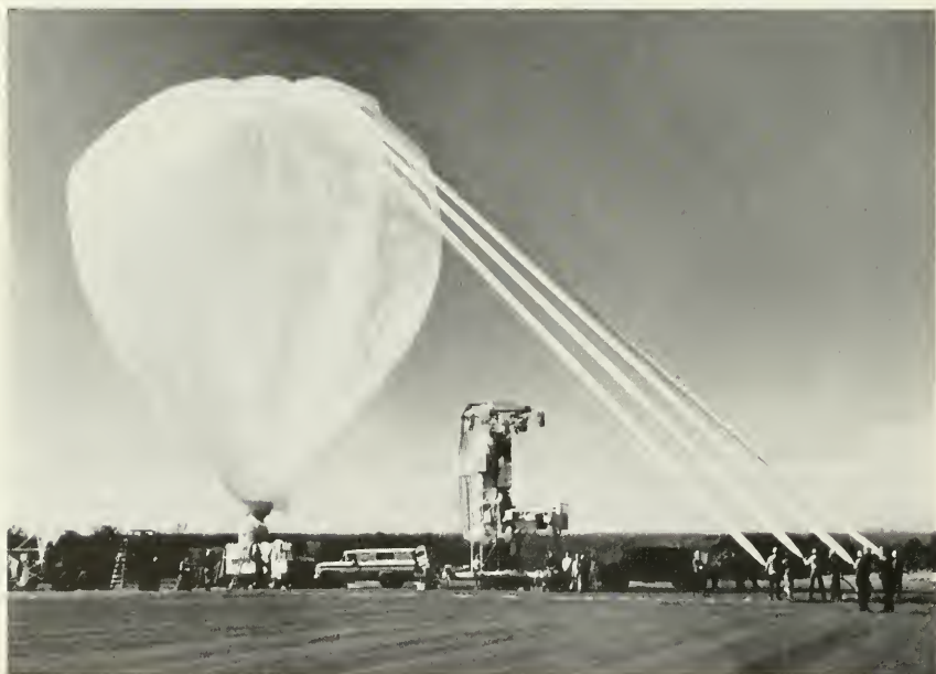
2. Inflation of the launch balloon. Stratoscope II is in the center of the photograph.
