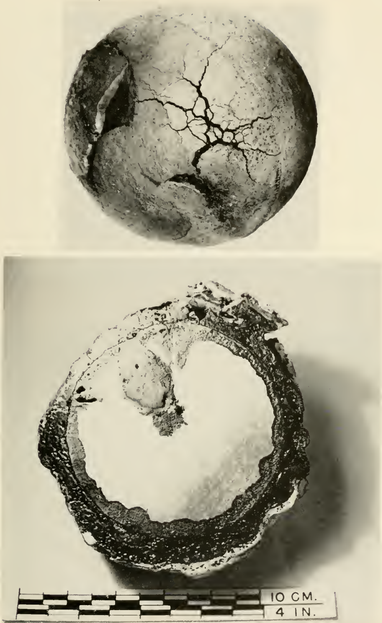
Several 6-pound cast-iron cannon balls were recovered from the wreck site of the H.M.S. Looe sunk in 1744 off Looe Key in the Florida Straits. The upper illustration shows the condition of one ball after removal of calcareous incrustations. The lower shows a cross section of another ball in which a lead plug had been employed to fill a hole in the casting. The iron core is surrounded with a thick rind of iron oxide but the lead is relatively unaffected. Courtesy Department of Armed Forces History, Smithsonian Institution.
