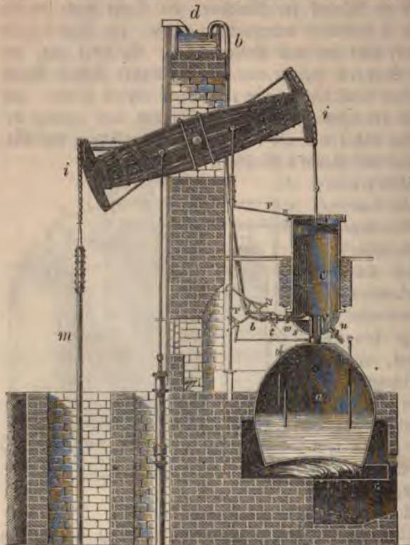
Fig. 392. Newcomen's Dampfmaschine.
