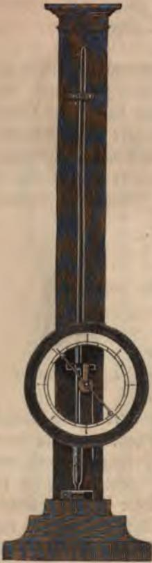
Fig. 88. Radbarometer.
