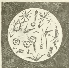
FIG. 3.—Microscopic Structure of Irichstone. A glassy base, with numerous feathered and needle-shaped microlites, and a sandstone crystal.
