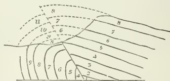
FIG. 30.—Inverted anticline and reversed fault.
