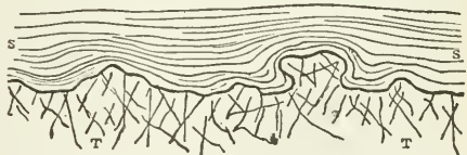
FIG. 57.—Section of the upper surface of an interbedded sheet T, showing how its unevenness are wrapped round and covered by the sedimentary rocks S.
