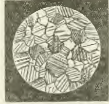
FIG. 5.—Microscopic Structure of Saccharoid white Marble (Carrara).
