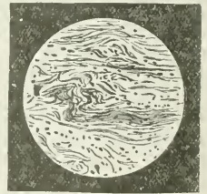
FIG. 2.—Microscopic Structure of Obsidian. A volcanic glass, with numerous microlites, which have been drawn out in a general direction during the flow of the melted rock (filio-structure). (X 18 diameter). In their most typical condition they consist entirely of a non-
