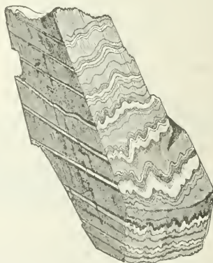
FIG. 64.—Sketch (by the late Mr Du Noyer) of a block of variegated slate from Devil's Glen, county Wicklow. The crumpled bands mark the bedding, and the fine perpendicular striæ in front are the cleavage planes; the fine lines on the darkened side merely represent shadon , and must not be taken for planes of division in the rock. It will be observed that the cleavage planes do not pass through the white bands.
