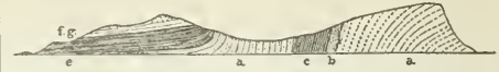
FIG. 20.—Section of the Isle of Wight—a monoclinical curve. a, Chalk; b, Woolwich and Reading beds; c, London clay; d, Bagshot series; e, Headon series; f, g, Osborne and Bembridge series.
