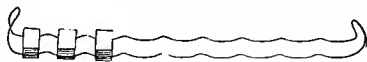
FIG. 46. A simple rack of bent wire suitable for the block-testing outlined in this study.
