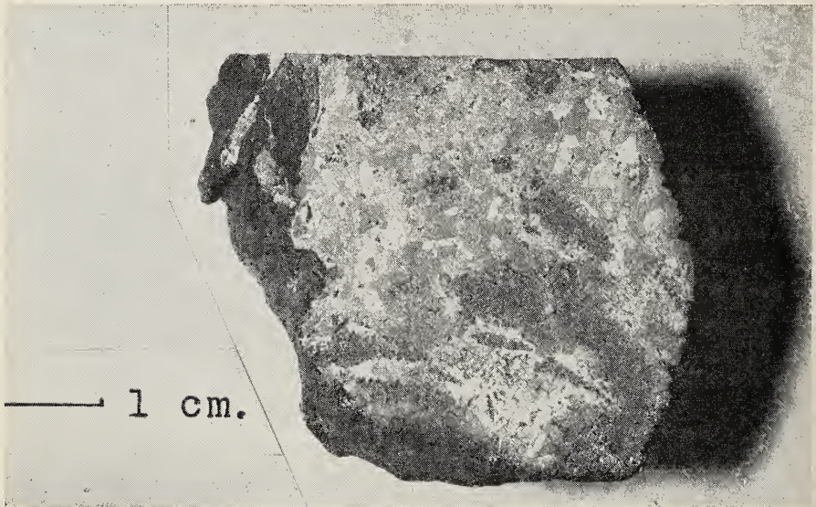
FIGURE 3. Etched surface of Saxeville specimen at the Milwaukee Public Museum, showing structure of the metal.
