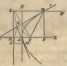
sa. This furnishes a very simple method of drawing a tangent to the parabola, when we know the abscissa of the point of tangency.
