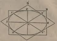
we conclude, that in the ellipse, the parallelogram constructed on any two conjugate diameters is equivalent to the rectangle on the axes.
