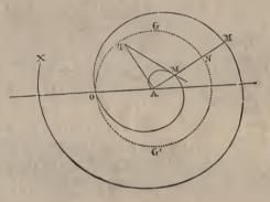
entire revolution, and at X at the end of the second revolution, and so on, the curve AMOM'X will be the spiral of Archimedes. From the nature of this generation, it follows that the ratio of the distance of each of its points from the point A to the line AO, will be equal to that of the arc passed over by the point O from the commencement of the revolution to the entire circumference; or, for any point M', we have the equation
