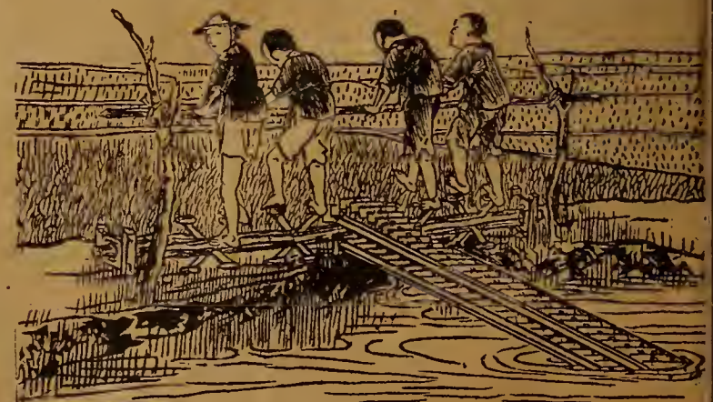
A Chinese device for drawing water from a pond into a rice field. It's pretty hard on feet
