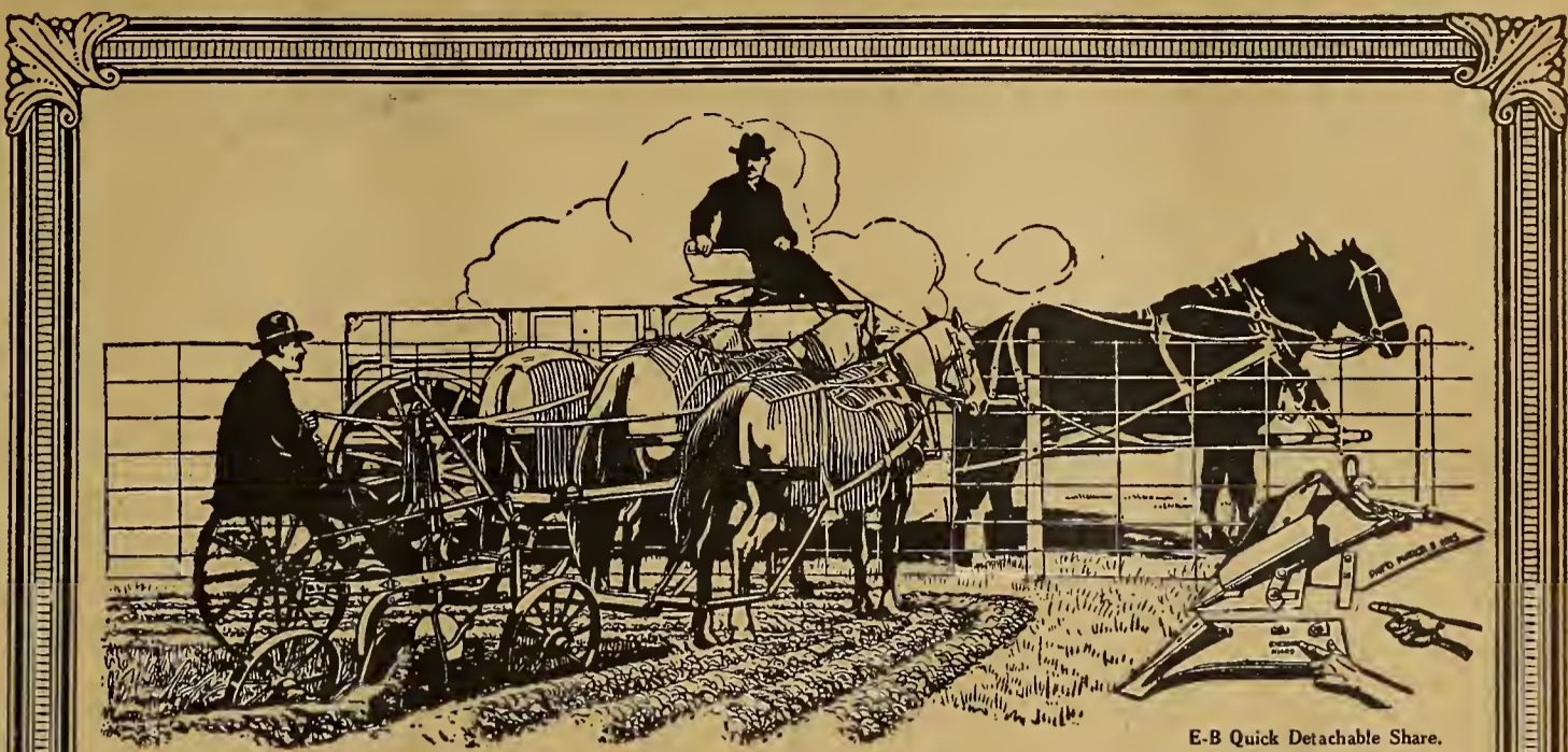
E-B Quick Detachable Share. One pull of lever forces share into position and locks it. No bolts. No wrench. Just your hands. Attached or removed in a few seconds.
