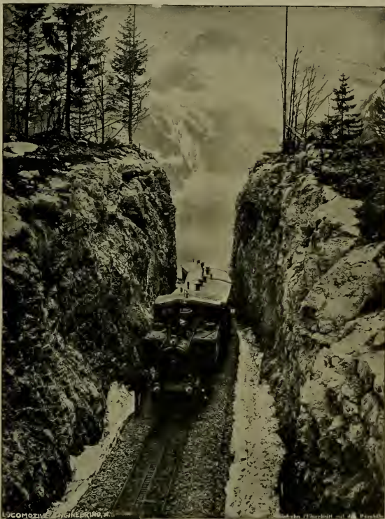
SUMMIT OF BRUNIG PASS, SWISS ALPS. GRADE 1 FOOT IN 10, OR 508 FEET PER MILE. ALTITUDE, 10,044 FEET.
