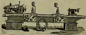
26 inch Triple Geared Lathe for Crank Pins and Driving Axles.
