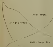
Boiler Gauge 128. M. E. P. 41.733 54.31 Miles per hour. Reverse lever in 2nd notch. Terminal open. Draft 30 ft. per M. E.
