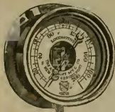
Locomotive Steam Gauge.
