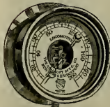
Locomotive Steam Gauge.
