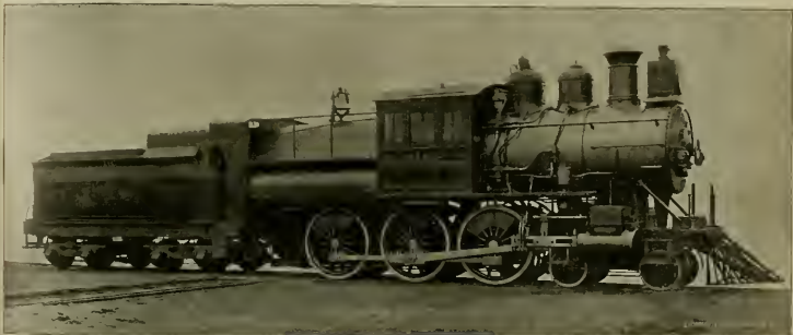
HEAVY TEN-WHEELER FOR MILK TRAIN SERVICE, D. L. & W. BUILT BY DAVID BROWN, M. E., AT THE COMPANY'S SHOPS, SCRANTON, PA.
