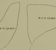
Boiler Gauge 128. M. E. P. 25.969 47.37 Miles per hour. Reverse lever in 2nd notch. Terminal open. Draft 30 ft.
