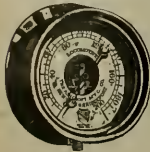
Locomotive Steam Gauge.
