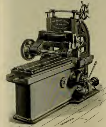
INGERSOLL 22X22 X 66-INCH MILLING MACHINE.
