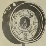
Locomotive Steam Gauge
