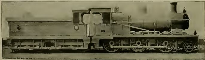
TWO-CYLINDER WORKSITE COMPOUND FREIGHT LOCOMOTIVE FOR ARGENTINE REPUBLIC BUILT BY NEILSON &amp; CO., GLASGOW, SCOTLAND.
