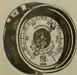
Locomotive Steam Gauge.
