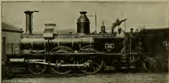
A GERMAN EXPRESS LOCOMOTIVE. OBSERVE THE GOSS STEEL AND HAND-HOLDS AND THE SUGAR-MILL CRANKS TO TENDERS-BRAKE.
