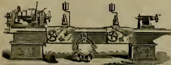
26 inch Triple Geared Lathe for Crank Pins and Driving Axles.
