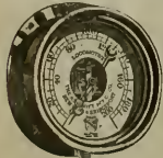
Locomotive Steam Gauge.
