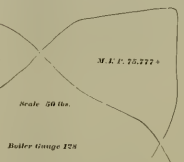
Boiler Gauge 128. M. E. P. 25.727 47.37 Miles per hour. Reverse lever in 2nd notch. Terminal open. Draft 30 ft.
