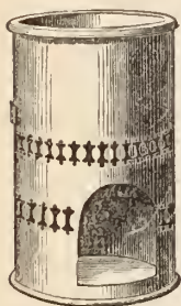
Fig. 11. Metallic tube, at the upper part of which the boiler is placed and at the lower part the lamp.
