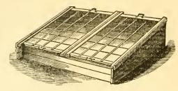
or several of any dimensions, the best of about three by seven feet. The back being higher than the front, gives a declivity to the sash, thus casting off the rain, which it would not do if flat.
