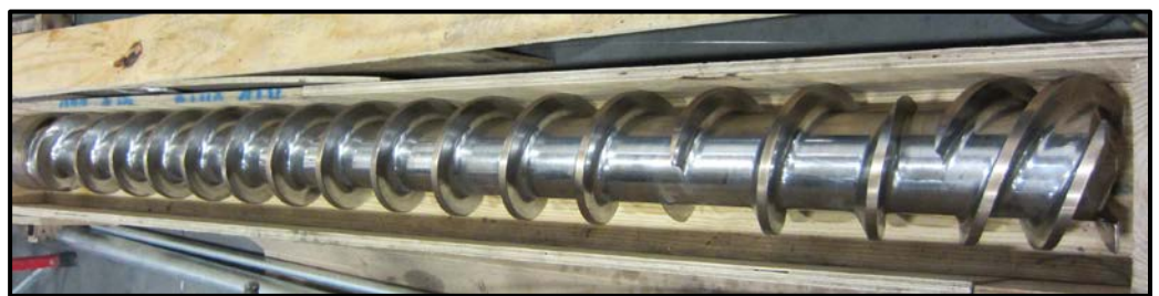
7.5 inch (190mm) diameter extrusion screw with bronze coated flights from DEMACO.
